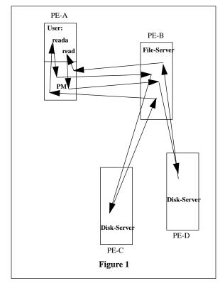
some time later is followed by a read() system call. Both calls are first processed by the local PM, are forwarded to a file server running on PE-B and finally processed by disk servers running on PE-C and PE-D.
