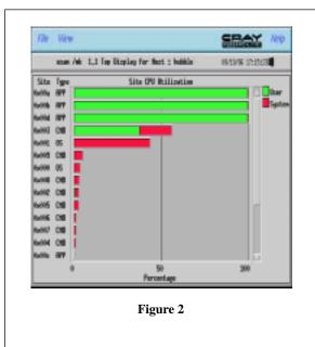
Display with three application nodes running 100% in user mode and one command and one support node running at non-trivial load levels.
