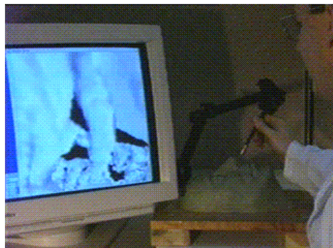
Figure 7: The Microscribe™ held by a surgeon inserted into the nasal cavity of a mock patient head. The monitor displays a view of the virtual patient in real time.
