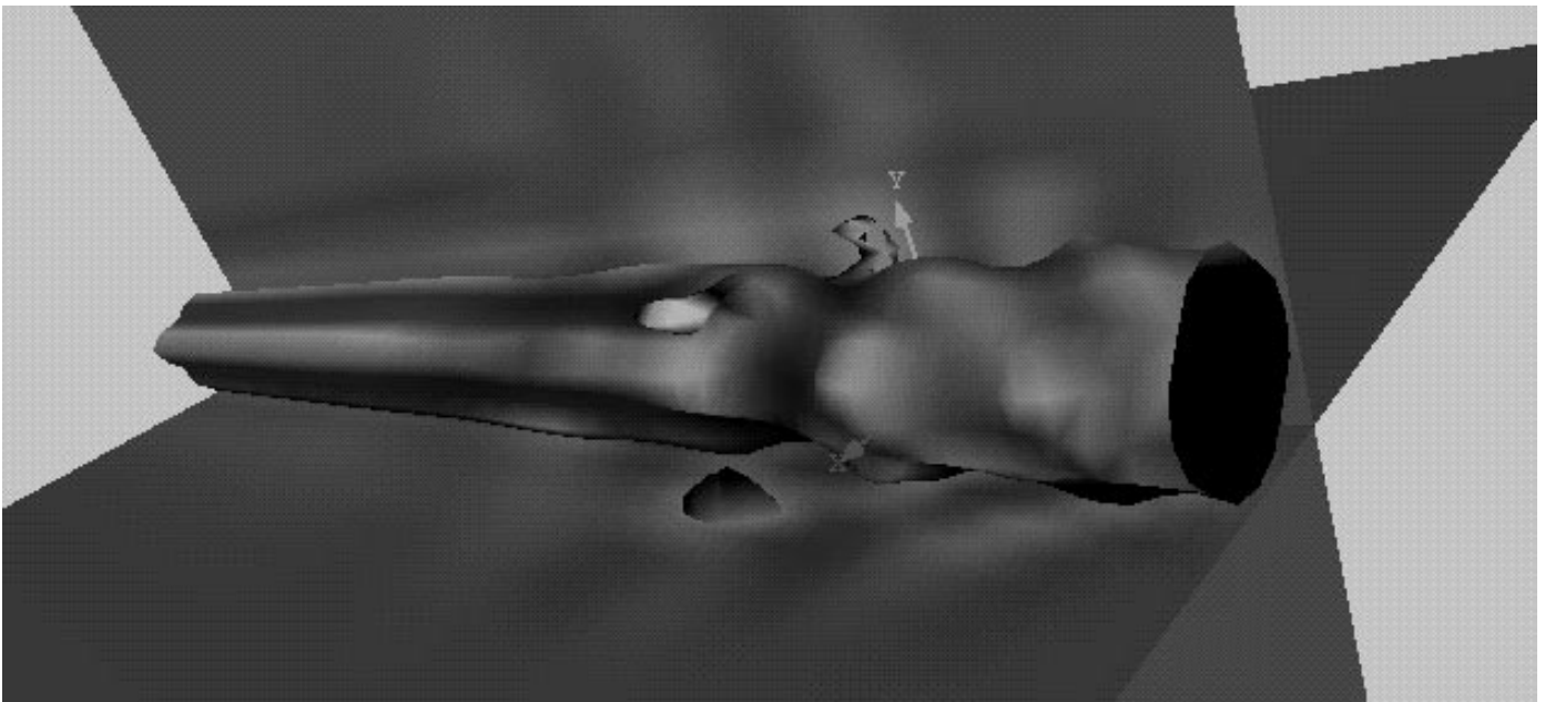
Figure 9: Simulation of a Vortex Breakdown by solving the 3D Navier Stokes Equations for an unsteady incompressible flow. Computation performed using Pegase from ONERA.
