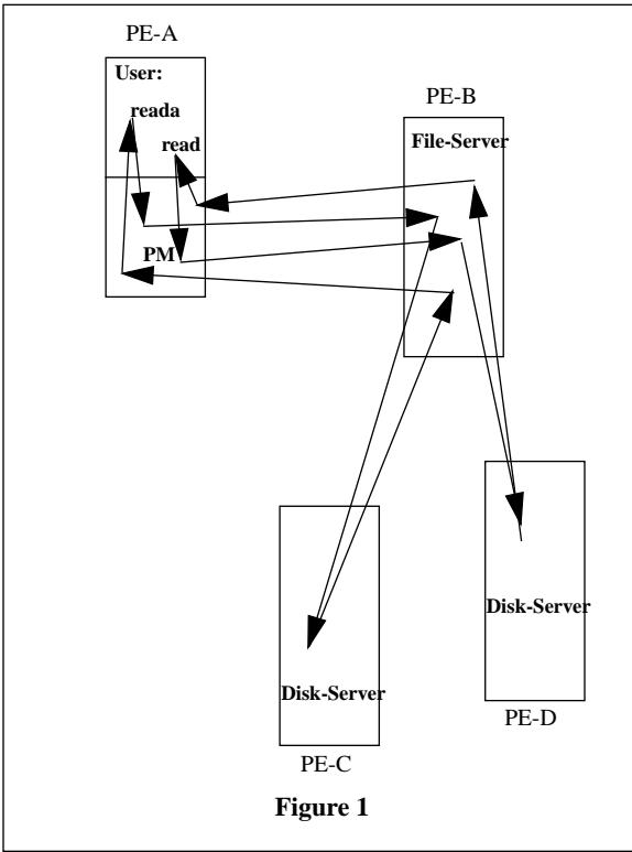
some time later is followed by a read() system call. Both calls are first processed by the local PM, are forwarded to a file server running on PE-B and finally processed by disk servers running on PE-C and PE-D.
