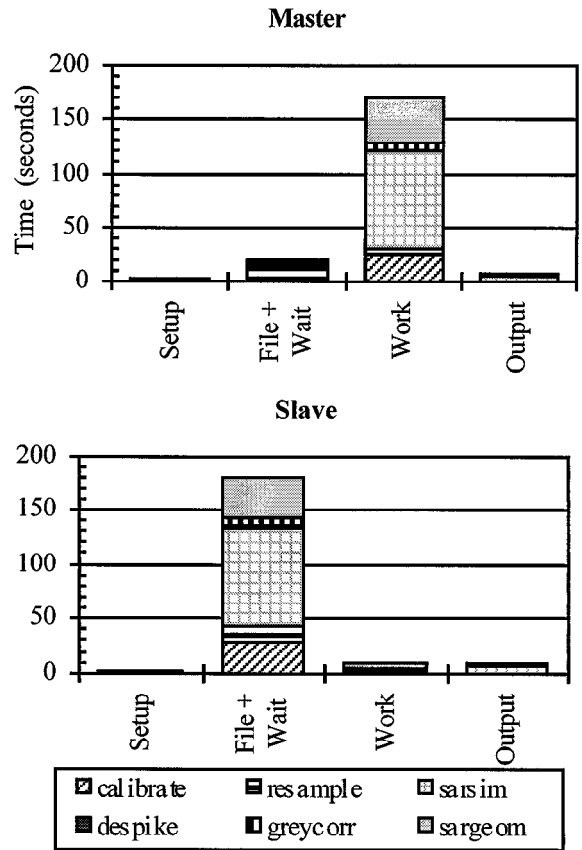
Figure 5: Example of sectioned timings using 16 T3D processors. Differences in master and slave tasks are immediately obvious, as are the large time portions used by calibrate , sarsim and sargeom .
