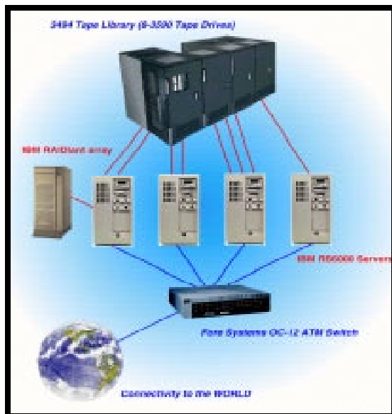
Figure 1. High Performance Storage System
