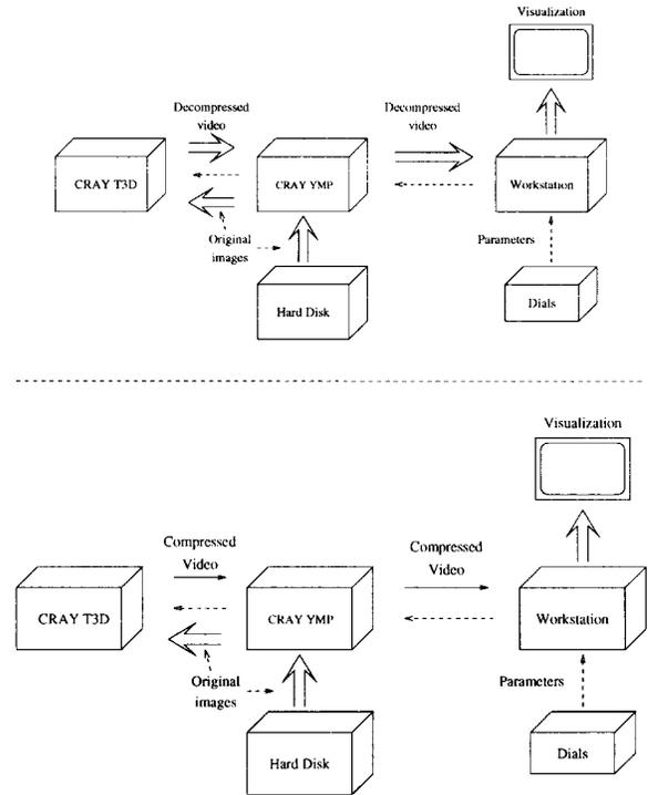
**Figure 1: Top: block diagram of *DirectView 1.0*. Bottom: block diagram of *DirectView 2.0*.**
