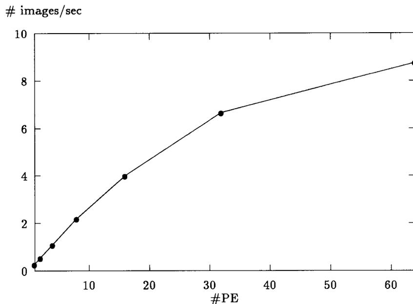
Figure 9: Number of processed images per second versus number of processors.
