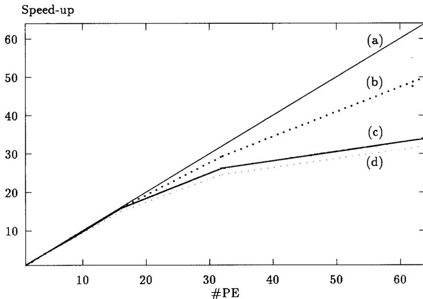
Figure 8: Speed-ups (*DirectView 2.0*). (a) Theoretical speed-up. (b) Speed-up of the compression algorithm only. (c) Speed-up obtained for the whole system, but without communication with the workstation. (d) Speed-up for the whole system.
