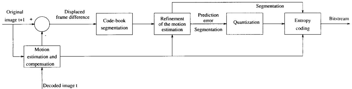
Figure 7: Simplified block diagram of the compression algorithm.
