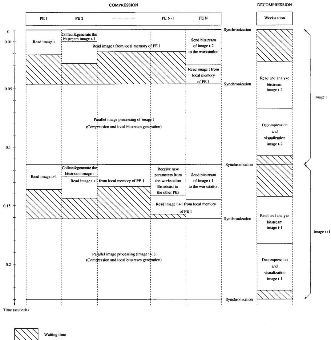
Figure 6: Load balancing representation (time measured for 64 processors)
