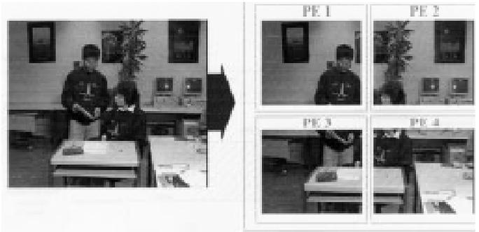
**Figure 5: Data partition for 4 processors**
