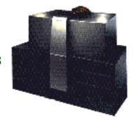
The CRAY T90 has extremely high memory bandwidth (880 GB/s peak) with great vector, gather, and random access to memory. It offers fast individual processors (1.8 GFLOPS peak) with very high bandwidth IO (Gbytes/second). Its UNICOS operating system is robust and provides excellent multijob throughput. It has proven high-performance for parallel applications, up to 32 processors.
