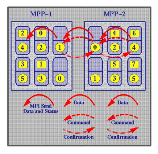
PACX provides an MPI\_COMM\_WORLD across the two machines involved. Numbers in the squares indicate node numbering as seen by the application in this communicator. If global node 6 wants to send a message to global node 2 the following steps are taken:
