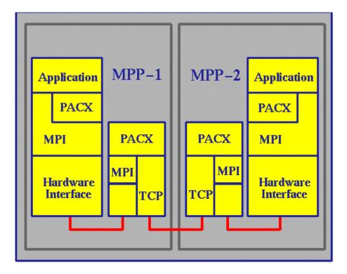
Communication via the network is done with TCP sockets. The concept of using two extra communication nodes (one for handling all outgoing communication and one for the incoming communication) has turned out to be a useful design as we plan to extend the concept to more than two machines. In addition it was easier this way to handle the complex communication needs of a real world application.
