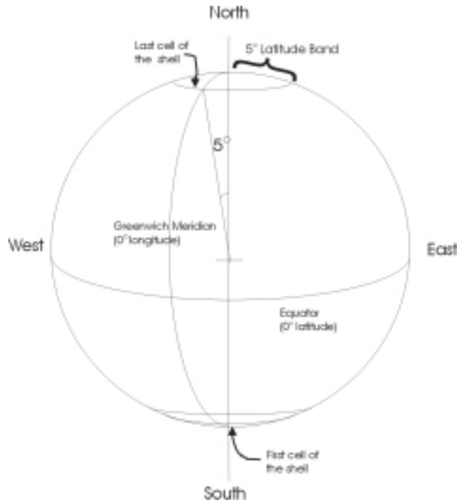
*fig 4: A schematic diagram to show how one shell of simulation cells are arranged.*
