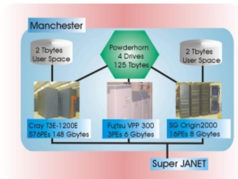
Fig 1: The CSAR cluster's configuration.
