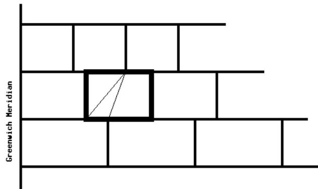
*Fig 7: A diagram showing the resampling scheme. It is the surface of a group of cells in 3 latitude bands projected in 2D. The cells appear rectangular, they are below the equator so each band has progressively more cells. We are looking at the cell with the thickened border, the thin line shows how it is cut into two triangular prisms and a trapezoid prism to make it curve with the bands above and below it.*
