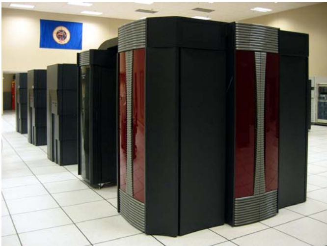
Figure 2. The production level Cray X1 LC (liquid cooled) machine following installation in the NCSI machine room for the AHPARC.
