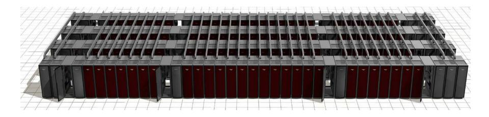
Red Storm is a supercomputer system leveraging over 10,000 AMD Opteron™ processors connected by an innovative high speed, high bandwidth 3D mesh interconnect designed by Cray
