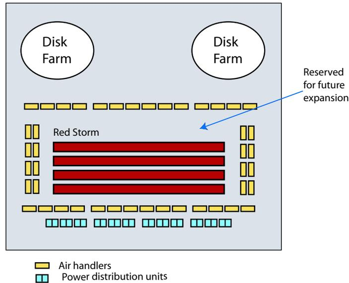
Figure 1: SCA equipment schematic
