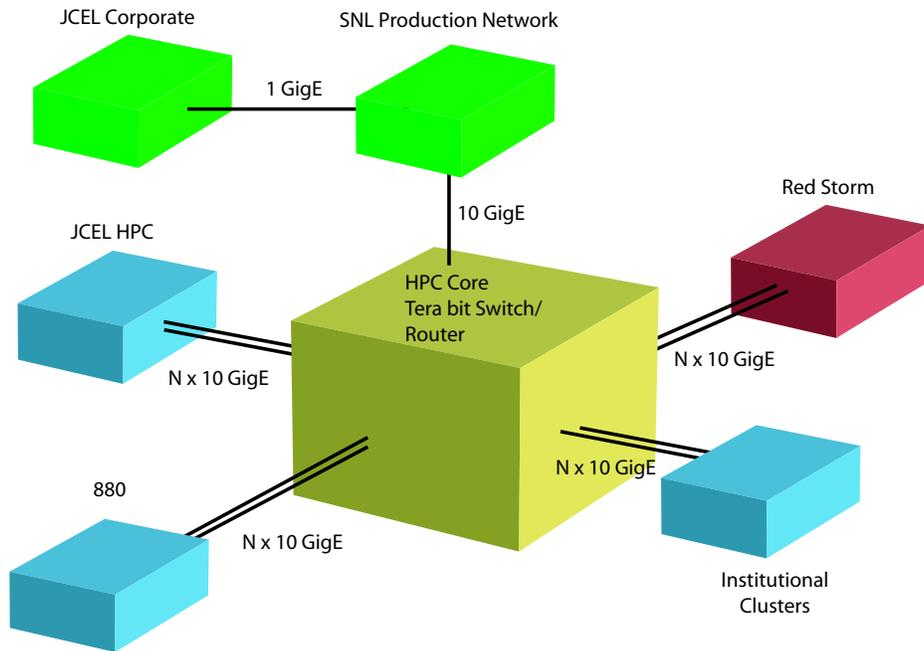
Figure 5: Sandia Backbone Network (Unclassified)
