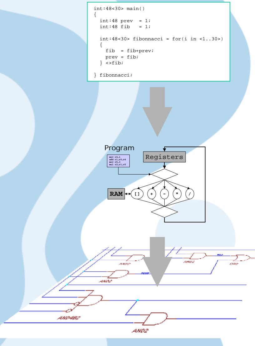
The traditional von Neumann processor is a state machine, operating instructions one at a time that are read from RAM memory.
