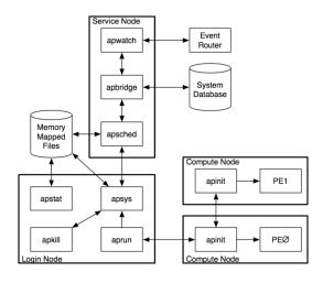
The ALPS software components communicate using the XML-RPC protocol. The protocol provides an extensible language that may easily be enhanced in future revisions of the software to support additional message types and services. In addition, ALPS makes use of memory mapped files to consolidate and distribute data efficiently. This reduces the demand on the daemons that maintain these files by allowing clients and other daemons direct
