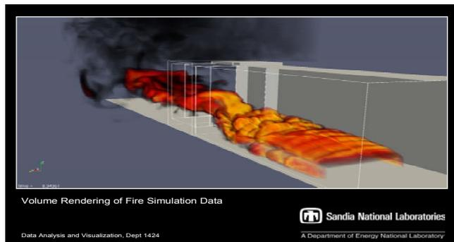
**Figure 2. Volume rendering of Fuego fire simulation data**
