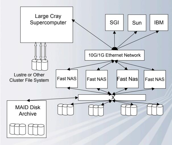
Add NAS storage for data sharing between Cray and other machines NAS backup and archive support •Long-term, managed data MAID for backup Separate storage networks for NAS and CFS stores •GridFTP, other software, for sharing and data migration
