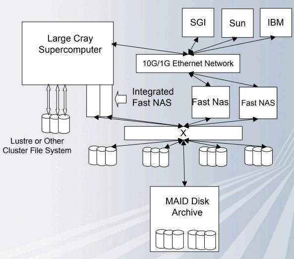
Integrate fast NAS with Cray network: reduced NFS overhead, compute node access to shared NFS store Single file system name space: all NFS blades share same name space internal and external MAID for backup and storage tier underneath NAS: FC versus ATA Separate storage networks for NAS and CFS
