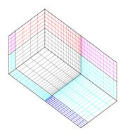
A ninety degree section of a solid cylinder with the center filled by two transition blocks of elements.
