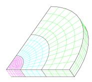
A 2D mesh consisting of nine material blocks that is transformed using a user supplied function.
