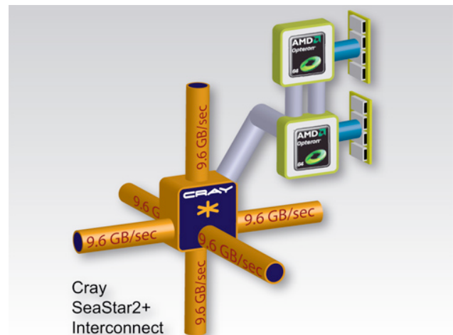
9.6-GB/sec-peak bidirectional network links in a 3D torus topology.
