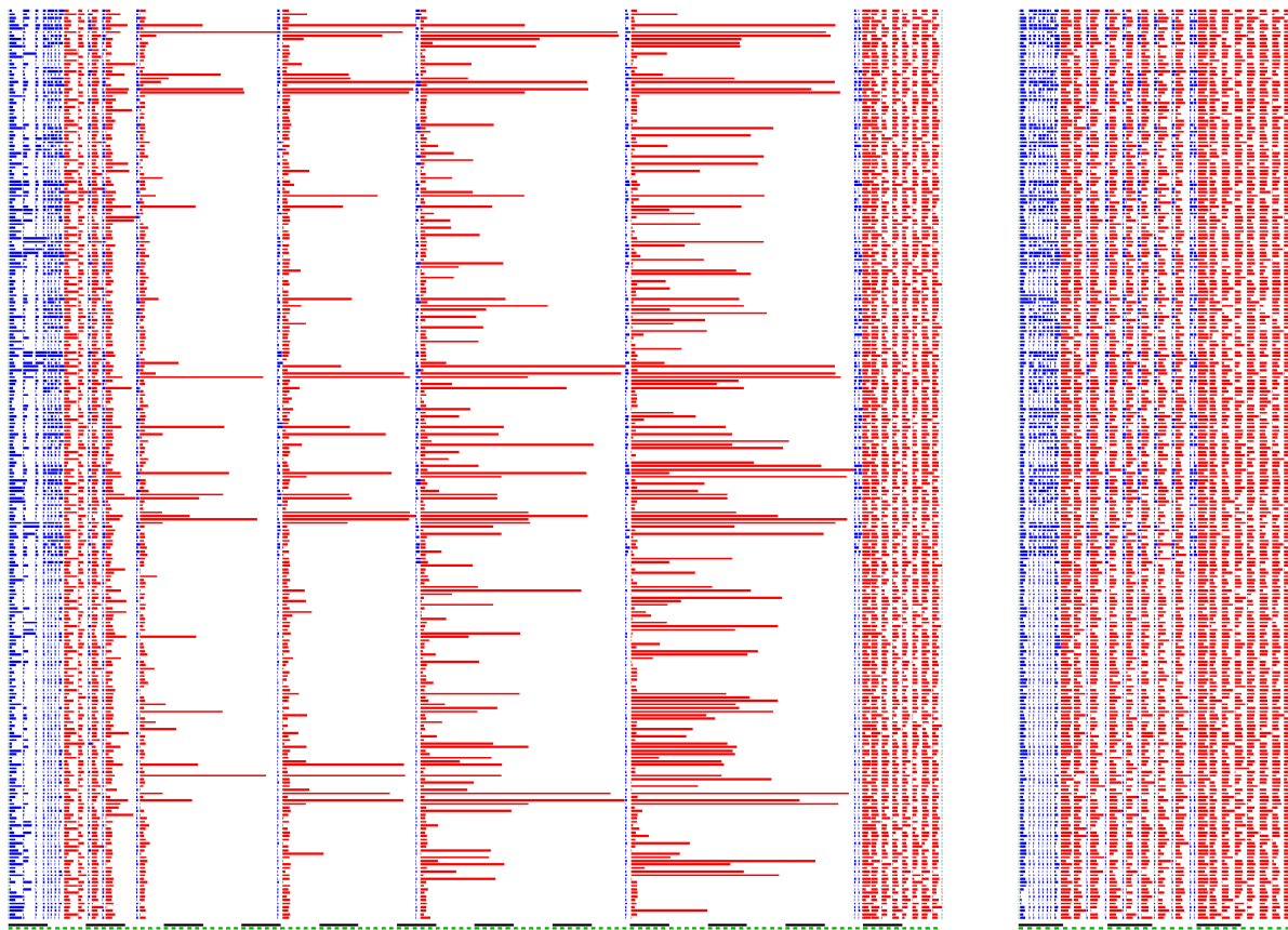
(a) Before: slow reads by a few processors force all processors to wait increasing the runtime of the application (b) After: slow outliers gone
