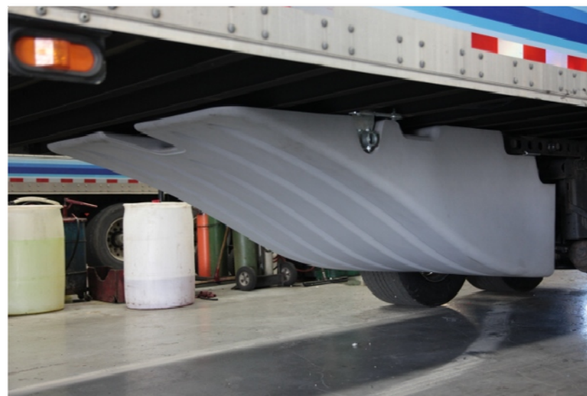
Trailers equipped with this front tray fairing and other BMI Corp. SmartTruck UnderTray components can achieve between 7 and 12 percent improvements in fuel mileage. (Photo courtesy of BMI SmartTruck)
