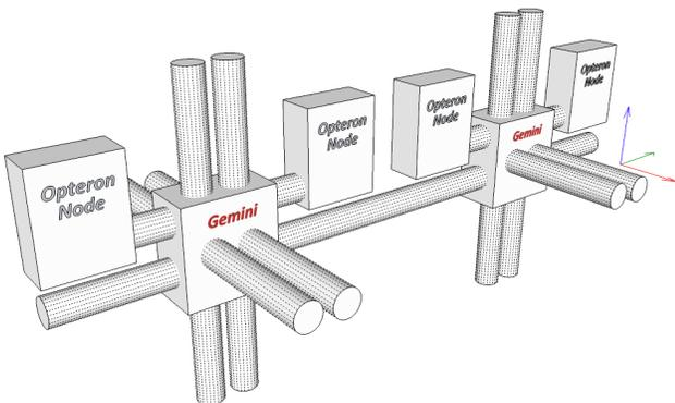
Fig. 1. High-level cartoon showing 4 Operton nodes connected by 2 Gemini ASICs. The X,Y, and Z axes are depicted as Red, Green, and Blue arrows, respectively.
