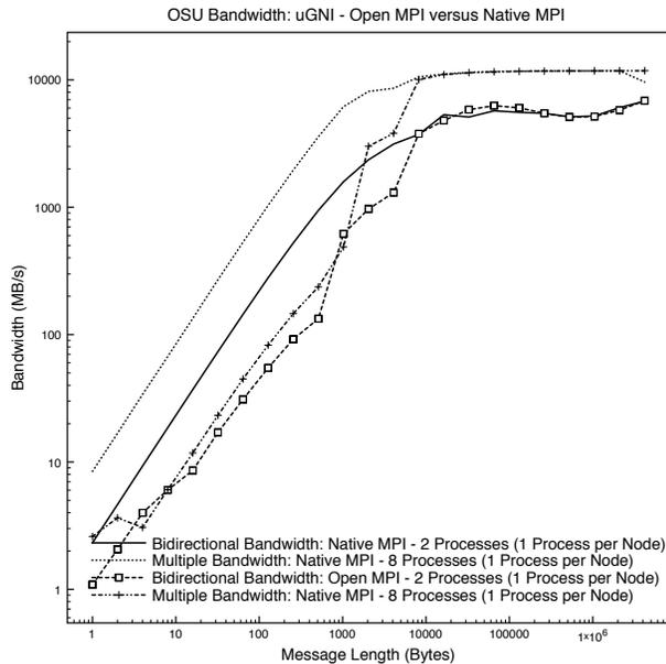
Fig. 6. Log-log plot showing uGNI bandwidths for 2 and 8 processes reported by OSU’s MPI micro-benchmark suite. Bidirectional bandwidth measured with *osu\_bibw* and multiple bandwidth measured with *osu\_mbw\_mr*.
