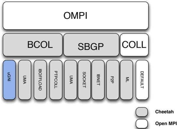
Fig. 2. Cheetah frameworks and components within Open MPI.
