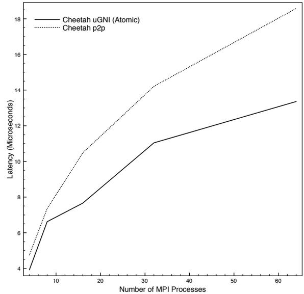
Fig. 7. Graph showing the performance of the Cheetah uGNI Barrier compared to the Cheetah p2p Barrier as a function of problem size.
