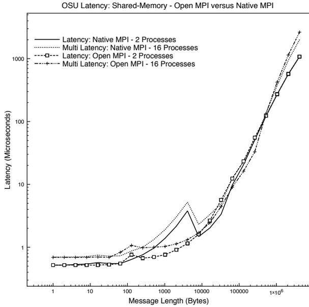
Fig. 3. Log-log plot showing shared-memory latencies for 2 and 16 processes reported by OSU’s MPI micro-benchmark suite. Latency measured with *osu\_latency* and multi latency measured with *osu\_multi\_lat*.
