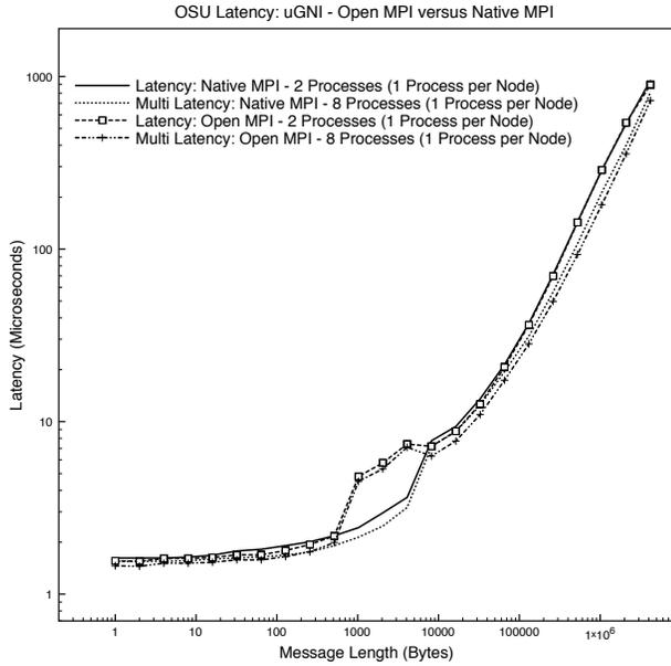
Fig. 5. Log-log plot showing uGNI latencies for 2 and 8 processes reported by OSU’s MPI micro-benchmark suite. Latency measured with *osu\_latency* and multi latency measured with *osu\_multi\_lat*.
