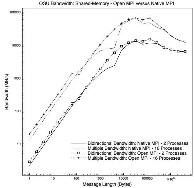
Fig. 4. Log-log plot showing shared-memory bandwidths for 2 and 16 processes reported by OSU’s MPI micro-benchmark suite. Bidirectional bandwidth measured with *osu\_bibw* and multiple bandwidth measured with *osu\_mbw\_mr*.
