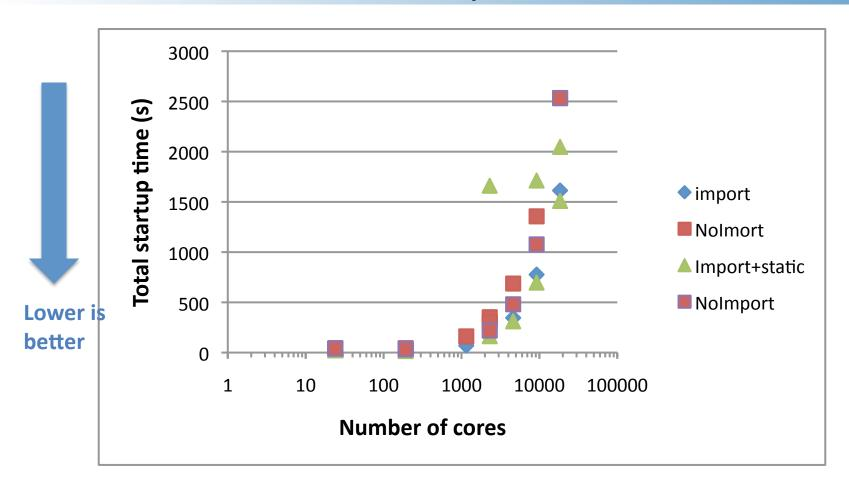
Statically linking MPI libraries to the pyMPI binary seems to help the total startup time of Warp.
