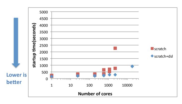
/scratch: all shared libs reside in the /scratch file system /scratch+dsl: user shared libs reside in /scratch, system provided shared libs in shared root file system (CRAY\_ROOTFS=DSL)
