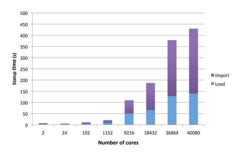
Warp users can run at their desired concurrency 40K within less than 7 minutes of startup time!
