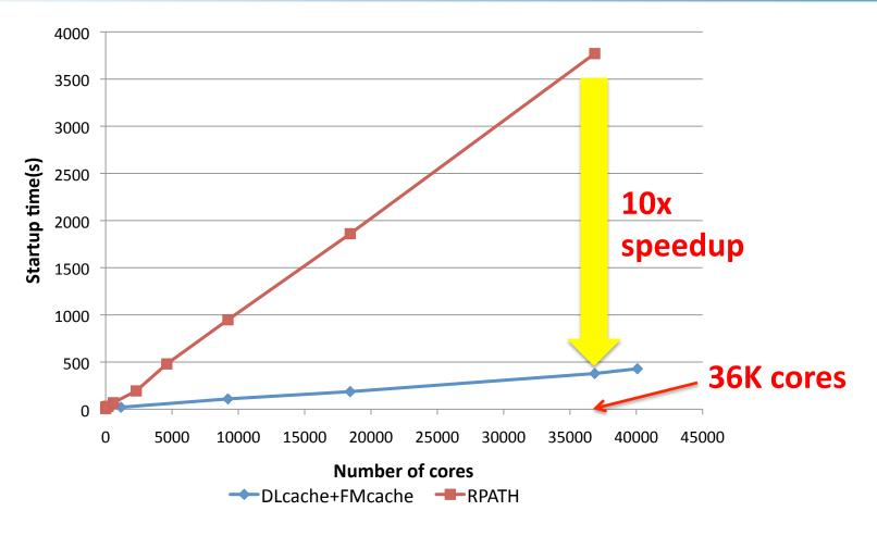
Warp startup time comparison to where we started with /scratch file system
