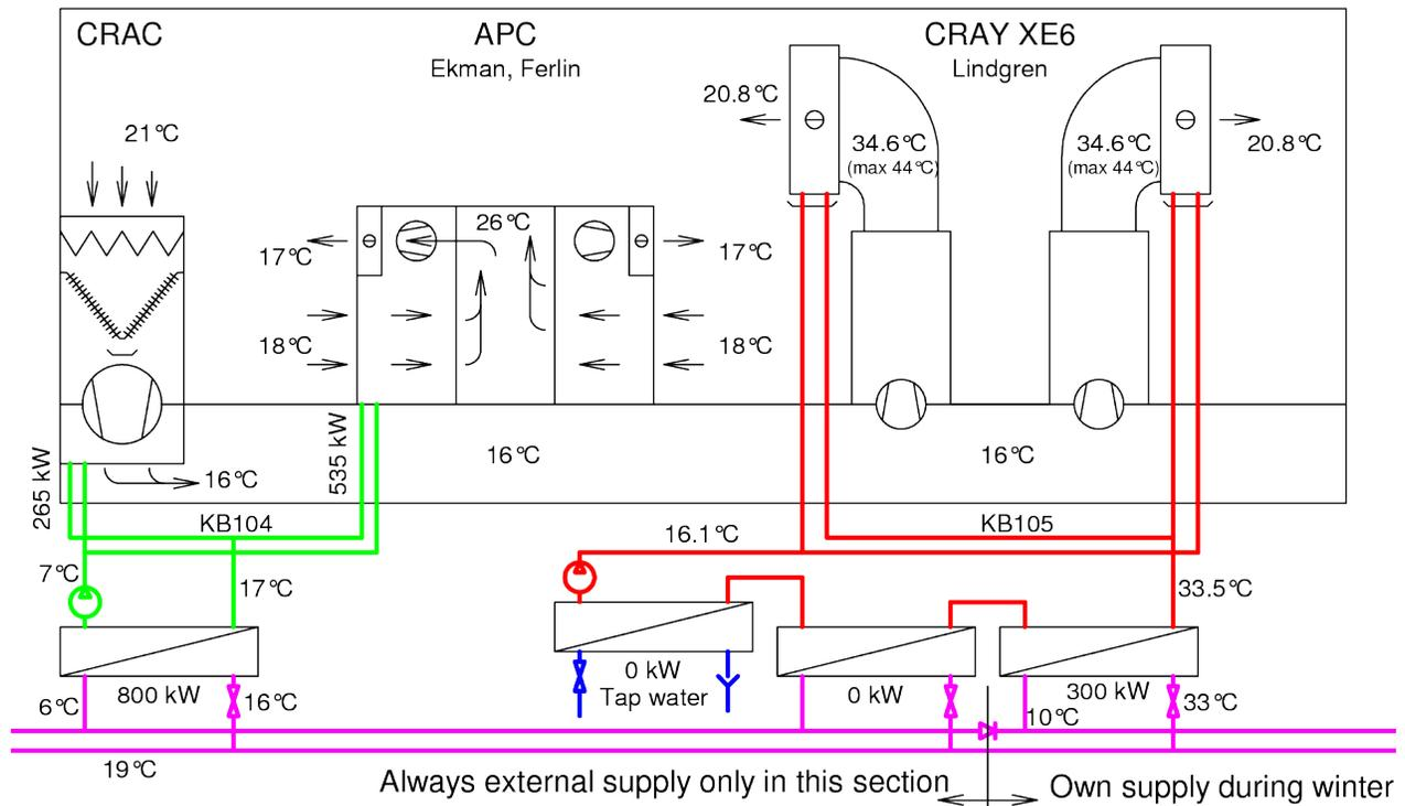
Figure 4. Layout of cooling in PDC: Ambient cooling via CRAC-units (left) and hot aisle APC connected via KB104 to district cooling (with back-up). Also seen is KB105 serving Cray racks with high temperature cooling downstream the check valve backed up by conventional district cooling and tap water cooling.
