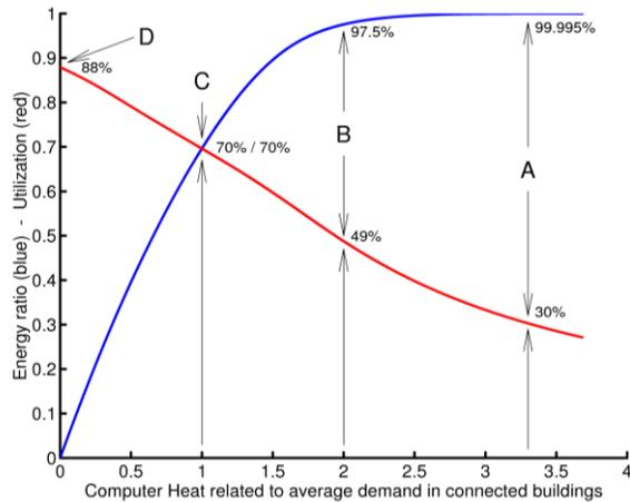
Figure 10. Heat re-use for Stockholm (1990-2010). The figure shows the variation in energy ratio (how much of the needed energy in the building is covered by re-used energy) and utilization (how much of the recovered energy is used in the buildings) depending of the size of the heat source.
