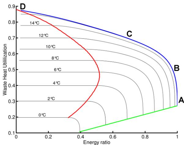
Figure 11. Variation in heat utilization depending on energy ratio when return temperature is limited by a fixed temperature. Blue line represents no limit.
