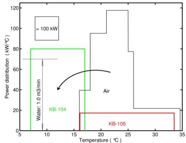
Figure 14. Cooling water temperature characteristics of computers at PDC. KB-104 is the district cooling circuit and KB-105 is the heat re-use circuit.
