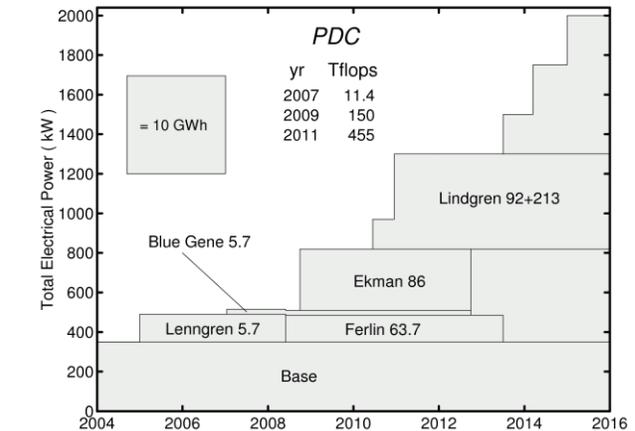
Figure 1. Power consumption at PDC.
