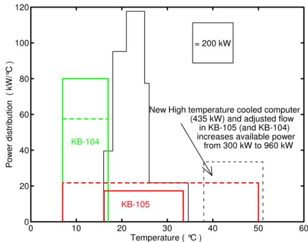
Figure 15. Increasing the amount of saved energy by connecting several computers with different temperature characteristics.
