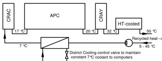
Figure 16. Heat sources at PDC connected in a chain.
