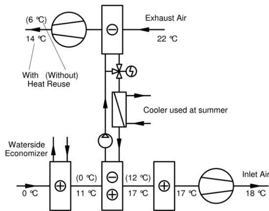
Figure 7. Current design in the chemistry building. Recycled water from the computer center pre-heats incoming air to the building.
