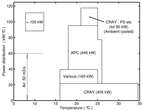
Figure 13. Cooling air temperature characteristics of computers at PDC.
