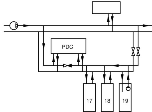
Figure 6. Ring shaped cooling system at the campus. The check valve closes and a self supplying section is formed once building 19 (the Chemistry building) is capable of taking care of all waste heat in the section. This happens at about 0 °C outdoor temperature. PDC uses coolant from both sides of the check valve.
