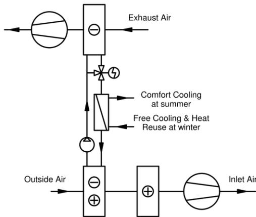
Figure 8. Suggested improved design in the chemistry building. This design doesn't need an additional heat exchanger.
