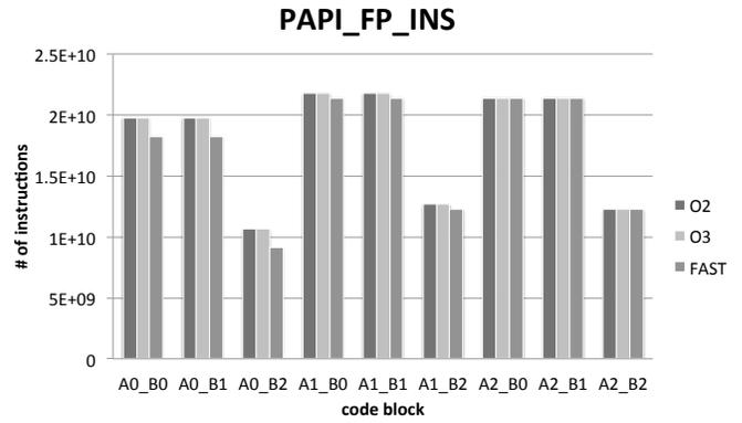
Figure 8. Number of floating point instructions for a 27k particle run
