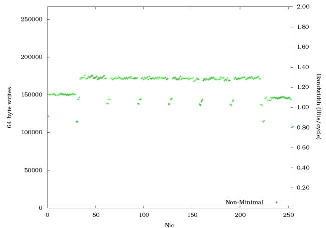
Figure 7: Number of 64-byte request packets transferred per NIC. Results are for 4 CTH traces per NIC with non-minimal routing
