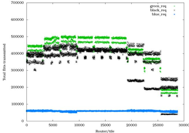
Figure 11 Number of flits transferred per port. Results are for CTH traffic with non-minimal routing.
