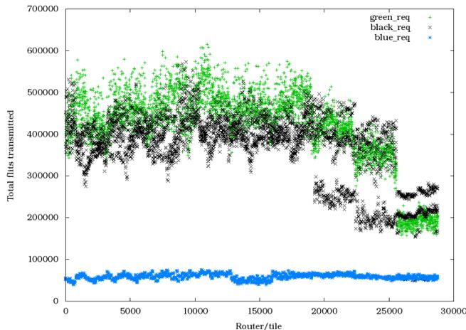
Figure 12: Number of flits transferred per port. Results are for CTH traffic with adaptive routing.
