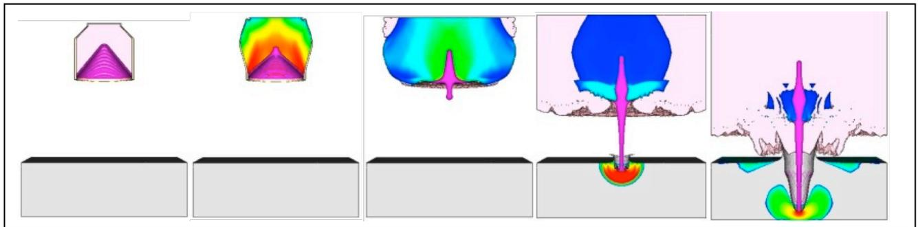
Figure 1: Sample output from CTH shaped-charge problem. The shaped-charge consists of a cylindrical container filled with high explosive capped with a copper liner. When the explosive is detonated from the center of the back of the container, the liner collapses and forms a jet which is shown striking a target.
