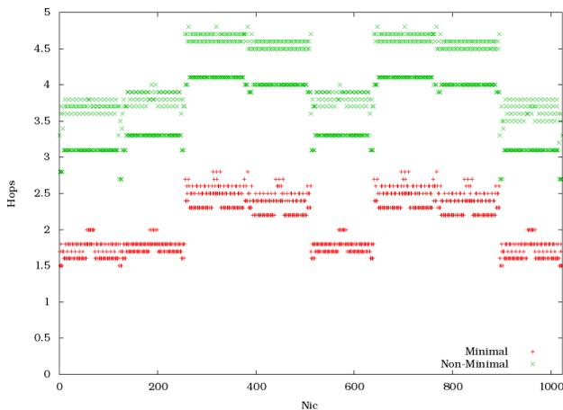
Figure 5: Initial CTH simulation results. Average hop count per NIC for minimal (red) and non-minimal (green) routing.
