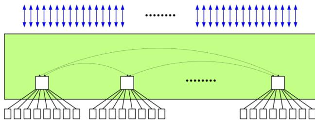
Figure 3: Electrical network connecting the nodes in a Dragonfly group. The optical links for each router (shown in blue) are pooled to form a single high-radix router.
