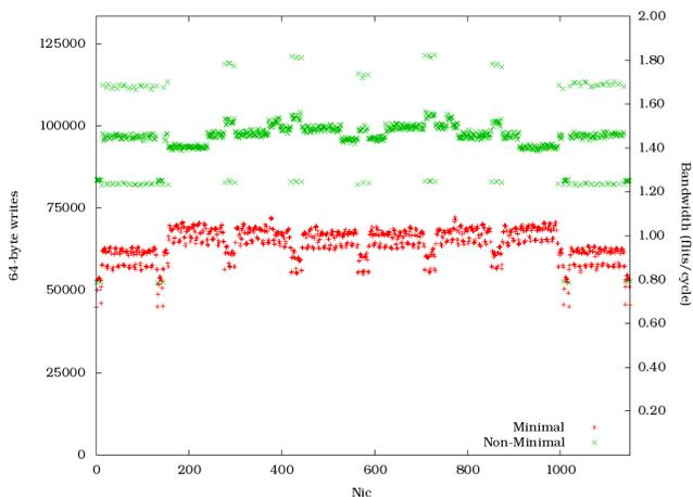
Figure 9: Number of 64-byte writes completed and equivalent bandwidth for synthetic CTH traffic. Results are for minimal routing (red) and non-minimal routing (green).
