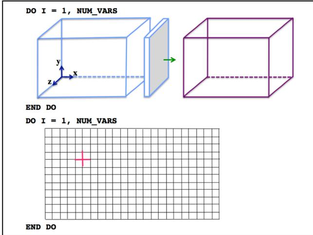
Figure 2: CTH bulk synchronous communication patterns. Each process exchanges face data with its neighbors on every timestep.
