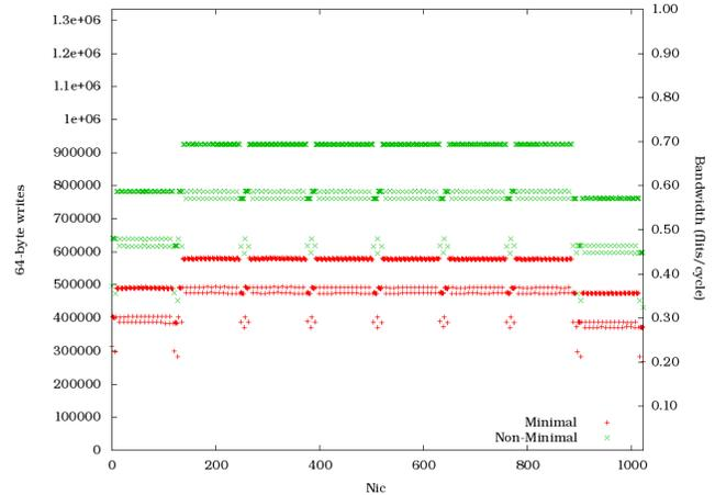
Figure 6: Initial CTH simulation results. Number of 64-byte writes completed per NIC for minimal and non-minimal routing.
