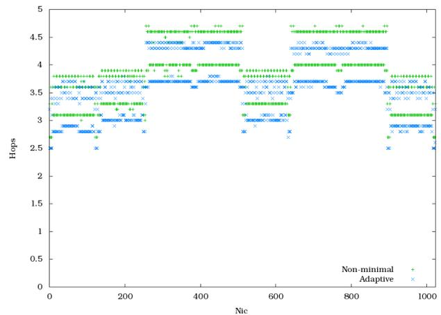
Figure 10: Hop count per NIC. Results are for trace based CTH traffic with non-minimal and adaptive routing.
