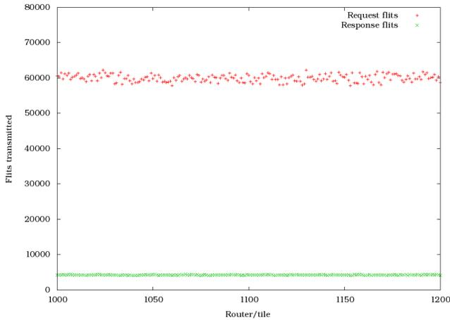
Figure 8: Number of flits transmitted by each optical link. Results are for CTH traffic with non-minimal routing.
