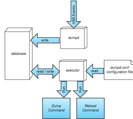
Figure 11. Dumpd Components and Interactions on the SMW
