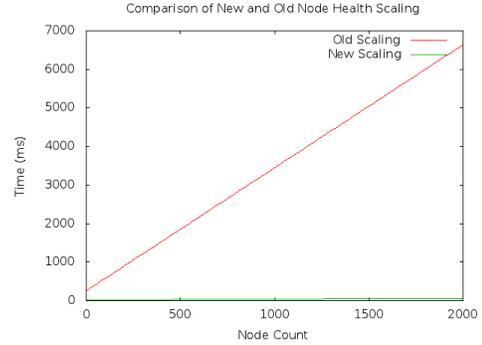
Figure 10. Comparison of old and new NHC scaling
