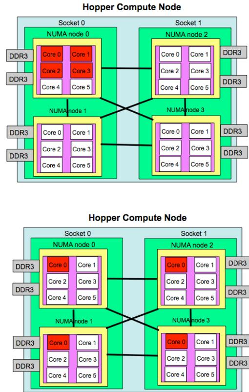
Figure 6. Illustration of the “-S” option in aprun. Upper: aprun -n 4 -d 6 ... Without “-S”, all 4 MPI tasks are allocated on the same NUMA node. Bottom: aprun -n 4 -S 1 -d 6 ... With “-S 1”, there is only 1 MPI task per NUMA node.
