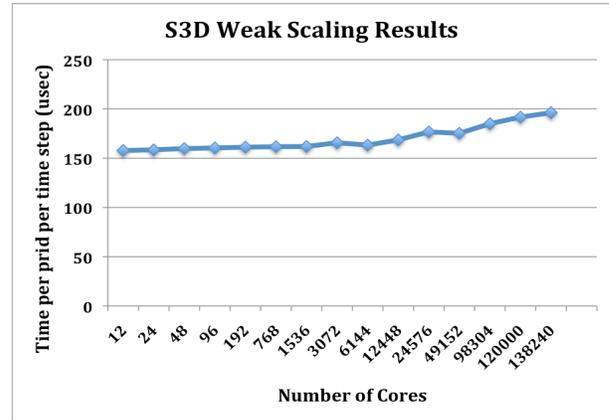
Figure 3. S3D run time per grid per time step using different number of cores on Hopper. This is weak scaling, so the ideal scaling is flat, and lower is better for scaling. 30x30x30 cube with c2h2 combustion chemistry. 50 time steps, no IO. (Courtesy of Hemanth Kolla and Evatt Hawkes)
