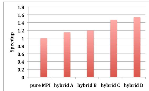
Figure 11. Speedup of MFDn with hybrid MPI/OpenMP implementations with overlapping communication and SpMV computations compared to pure MPI implementation. (Courtesy of H. Metin Aktulga *et al.*)
