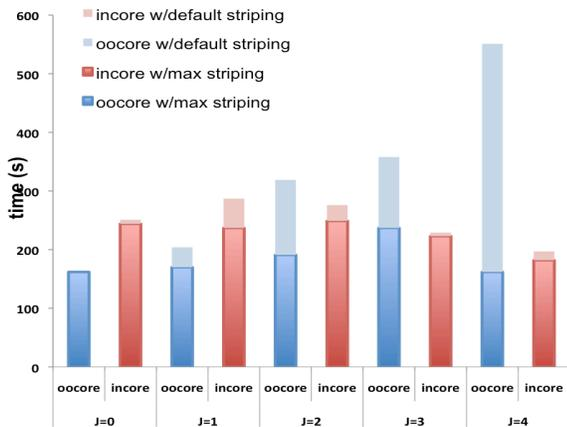
Figure 14. J-Scheme MFDn overall run time (computation plus IO) with out-of-core and in-core implementations using default and max file stripings. (Courtesy of H. Metin Aktulga *et al.*)
