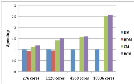
Figure 10. Speedup of MFDn with different numbers of total processors using different MPI rank orderings. BCM ordering is the best. (Courtesy of H. Metin Aktulga *et al.*)
