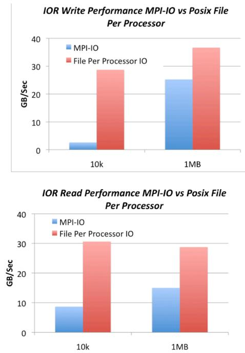
Figure 13. IOR write (top) and read (bottom) performance MPI-IO vs. Posix file per processor using different block sizes on Hopper scratch Lustre file system. (Courtesy of Yushu Yao)
