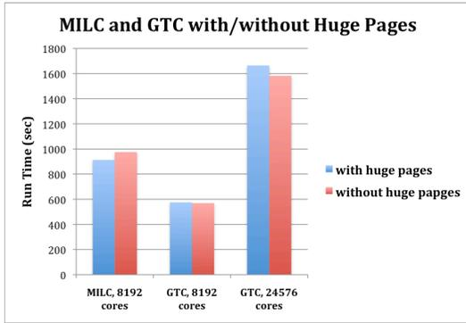
Figure 12. Run time of NERSC benchmarks MILC and GTC with and without huge pages. GTC 8,192 core and 24,576 core runs used different problem sizes.
