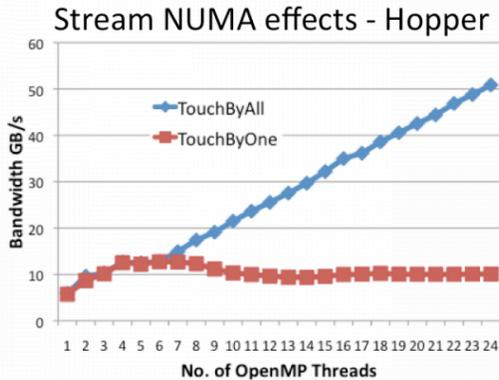
Figure 5. NUMA effects on Hopper with the STREAM benchmark. The result shown here is from a single node, with pure OpenMP, using 1 to 24 threads. (Courtesy of Hongzhang Shan)
