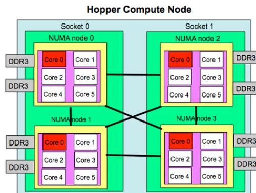
Figure 1. An illustration of a Hopper compute node. There are 4 NUMA nodes per node, and 6 cores per NUMA node. Memory access to a remote NUMA domain is slower than within the local NUMA domain.
