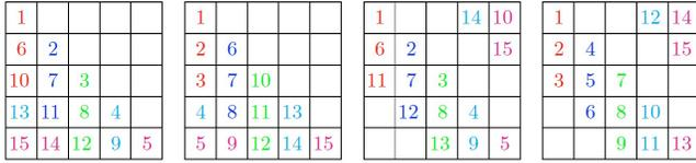
Figure 9. Illustration of 2D decomposition of the Hamiltonian H over processors in various rank orderings. Total of 15 processors (5 diagonal processors) in this case. From left to right: Diagonal Major (DM) ordering, Column Major (CM) ordering, Balanced Diagonal Major (BDM) ordering, and Balanced Column Major (BCM) ordering. (Courtesy of H. Metin Aktulga *et al.*)
