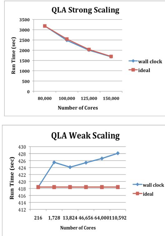
Figure 8. Scaling of Qutatum Lattice Gas Algorithm. Top: strong scaling. Bottom: weak scaling. The problem sizes used for the strong scaling and weak scaling are different. (Courtesy of Min Soe).
