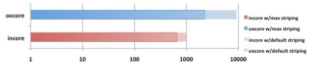
Figure 15. J-Scheme MFDn run time with out-of-core and in-core implementations using default and max file stripings for a larger problem size. Top: Computation and IO time with default striping. Bottom: Total run time with default and max stripings. (Courtesy of H. Metin Aktulga *et al.*)
