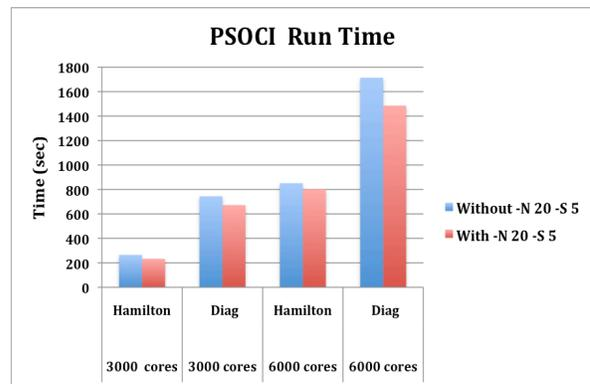
Figure 4. PSOCI run time with and without using fewer cores per node. 3,000 core and 6,000 core runs used different problem sizes. (Courtesy of Jeffrey Tilson)
