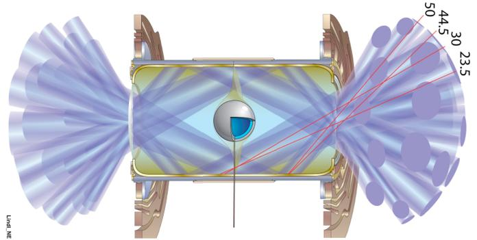
Fig. 1: The figure shows the laser beams entering the hohlraum through holes in both ends and propagating through the plasma until they reach the hohlraum wall. The hohlraum is a can-like object used to trap the x-rays emitted by the hot interior walls of the hohlraum.
