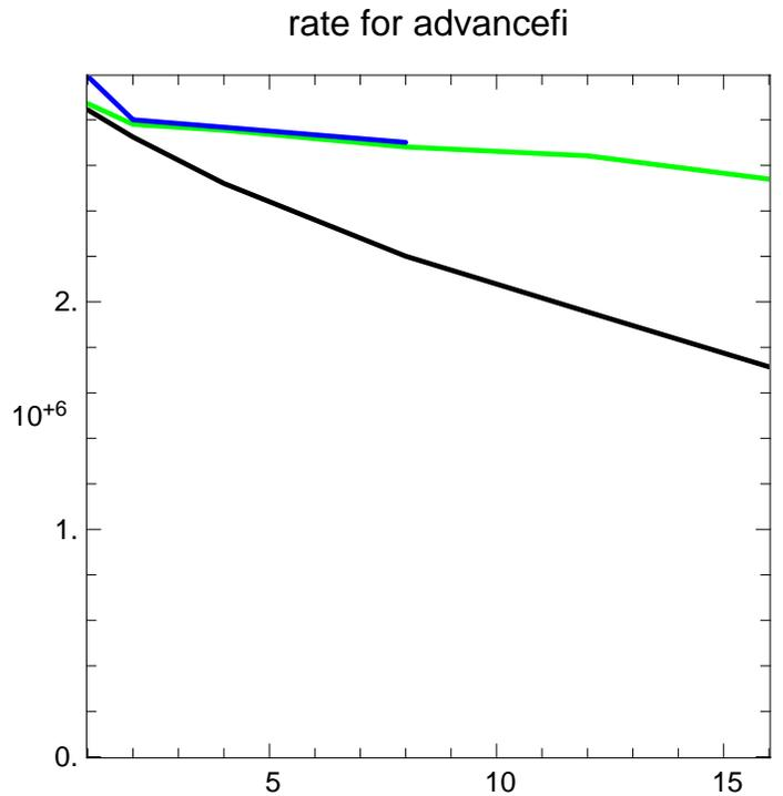
Fig. 7: The figure shows the zones updated per second per core for the advancefi kernel on a Sandy Bridge processor as a function of the number of threads. Weak scaling (green) and hybrid scaling (blue) have times nearly independent of the number of threads. The performance drops significantly in the strong scaling study (black).
