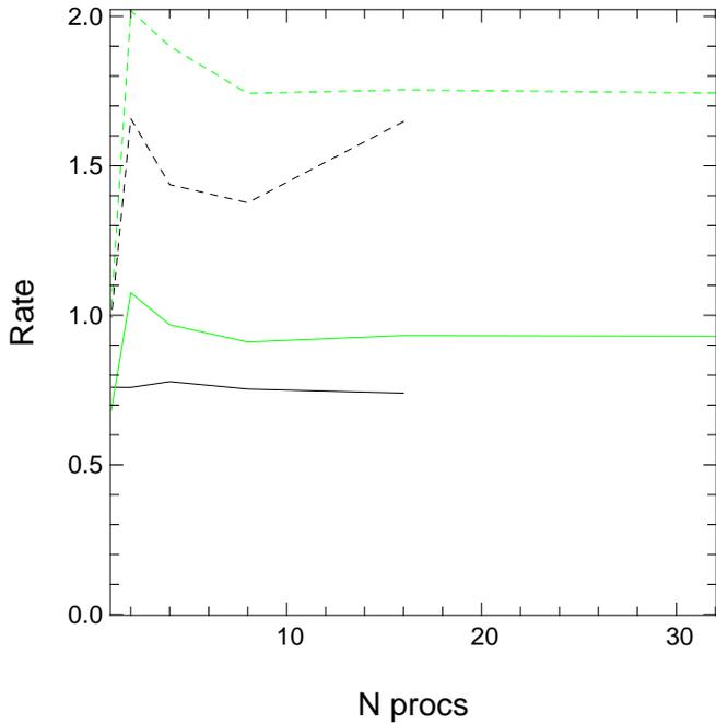
Fig. 9: The figure shows the rate (averaged over threads) at which zones are updated per core as a function of the number of processes for the couple4 kernel on an Intel Sandy Bridge processor. Solid lines are for the non-SIMD version and dashed lines for the SIMD version of the couple4 kernel. The black lines are for one thread per core and the green lines are for two threads per core. The zones per core are the same for all runs.
