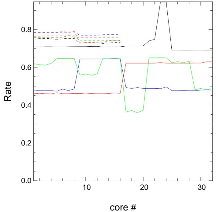
Fig. 10: The figure shows the rate at which zones are updated per core for the couple4 kernel on Intel Sandy Bridge (dashed lines) and AMD Interlagos (solid lines) processors. Black is 16 processes with 1 thread each, green is 8 processes with 2 threads each, blue is 4 processes with 4 threads each, and red is 8 processes with 2 threads each. The rates for the Interlagos chip are for a floating point unit and its two associated integer cores.
