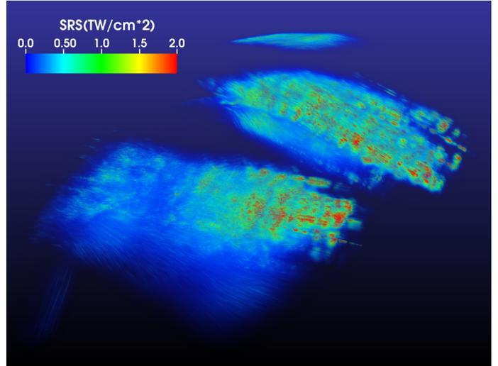
Fig. 12: The figure shows the SRS backscattered light at a time shortly before the peak of the first burst. The SRS from the two beams is spatially separated at this time. Later on there is SRS in the region where the two beams overlap.
