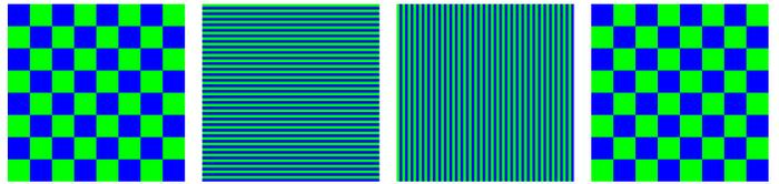
Fig. 3: The 2D FFT message passing scheme. MPI\_Alltoall is used to transpose from a checkerboard decomposition, to decompositions by rows and columns, and back to a checkerboard. The FFTs are performed while the data is in rows or columns.
