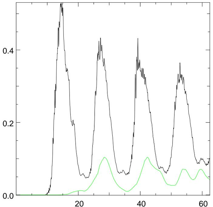
Fig. 13: The figure shows the SRS and SBS backscattered light as a function of time. The scattered light is shown as a fraction of the incident light.
