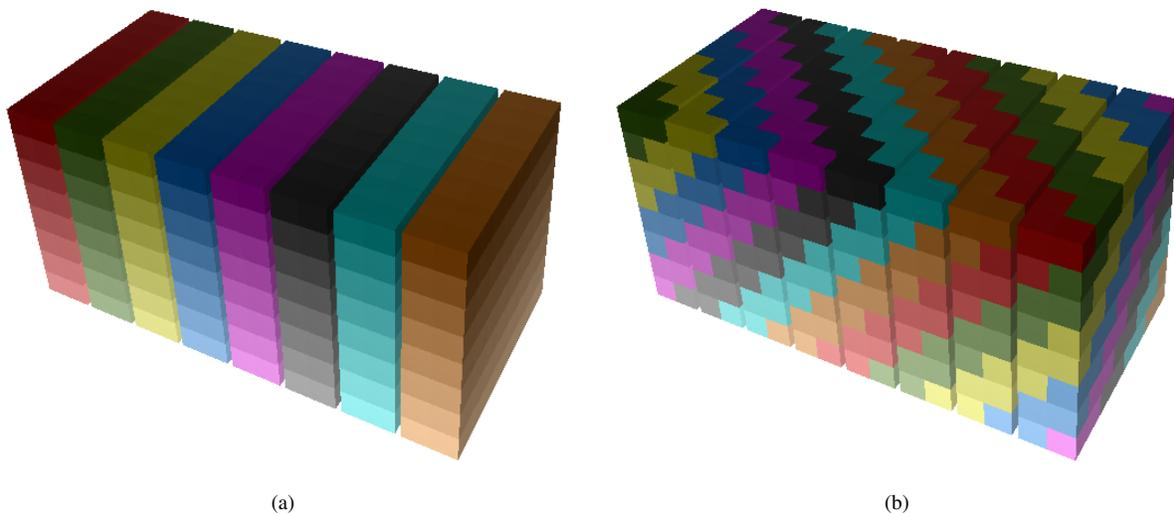
Fig. 5: This figure shows how a simple partitioning of the BG/P torus can be turned into a tilted mapping. (a) The 8x8x8 partition has been divided into 8 slabs. Each slab corresponds to an xy-slab in physical space. (b) The slabs have been tilted in two directions. The mapping connects an xy-slab in physical space to a tilted plane on the interconnect. Messages passed within an xy-slab can use all three link directions with this mapping, producing a higher message passing rate.
