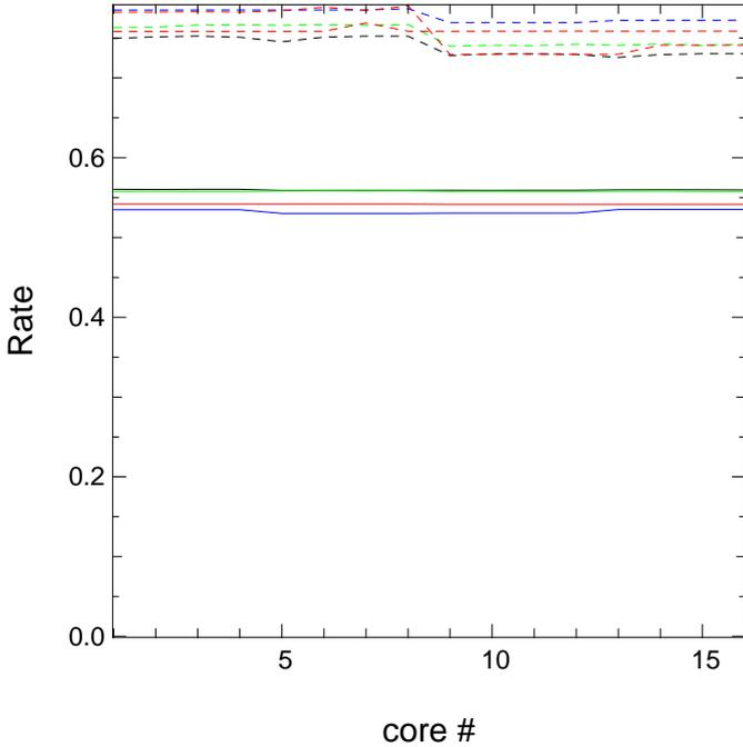
Fig. 11: The figure shows the rate at which zones are updated per core for the couple4 kernel on Intel Sandy Bridge (dashed lines) and AMD Magny Cours (solid lines) processors. Black is 16 processes with 1 thread each, green is 8 processes with 2 threads each, blue is 4 processes with 4 threads each, red is 8 processes with 2 threads each, and magenta is 16 processes with one thread.
