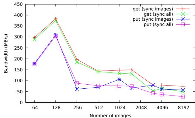
Figure 6. Performance of 3D halo swaps for  $100 \times 100 \times 100$  local arrays
