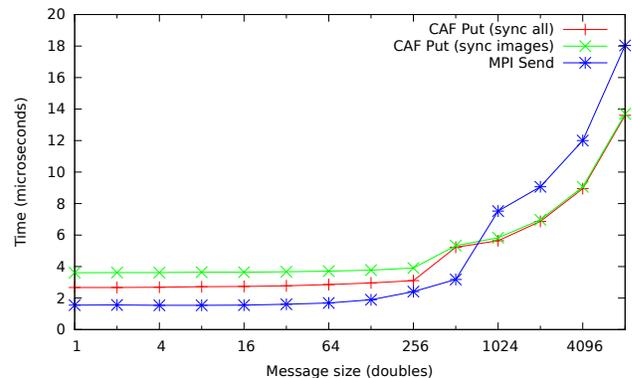
Figure 1. Latency of point-to-point data transfer using coarrays (with `sync all` and `sync images`) and `MPI_Send`
