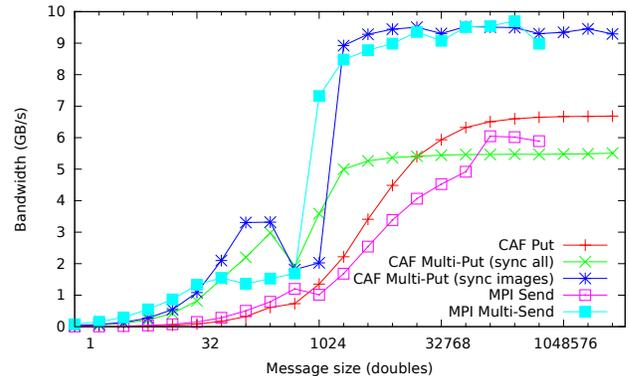
Figure 3. Bandwidth of single and multiple point-to-point data transfers using coarrays and `MPI_Send`
