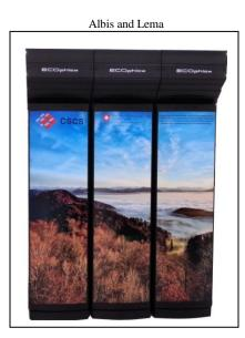
MeteoSwiss purchased a three-cabinet system from Cray, which is made up of XE6 hardware with AMD twelve core Magny-Cours processors and the Gemini network.
