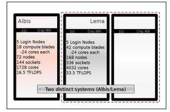
products and runs its calculations. This partition contains 5 login nodes and 18 compute nodes.
