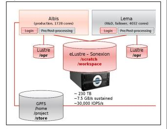
Both Albis and Lema have their own internal Lustre filesystems. MeteoSwiss requires five login nodes, with the rest of the service nodes being dedicated to SLURM, DVS and lnet routers. This leaves only 2 service nodes available for the Lustre servers. The main production data is fed from observational sites around Switzerland via a proxy to Albis, and is then copied via an rsync to Lema throughout the day.
