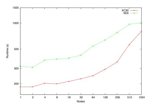
The benchmark compares the performance on the Cray XC30 versus the Cray XE6 of the hybrid OpenMP/MPI Gromacs 4.6, running with 16 MPI tasks per node and 2 OpenMP threads per MPI task.
