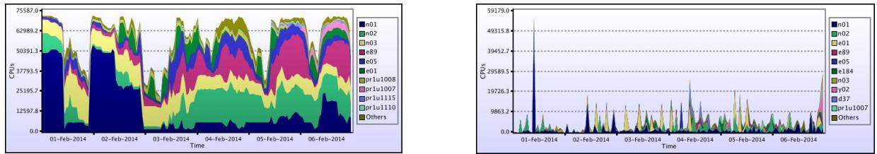
Figure 1. A comparison of CPU plots with and without overlap mapping. The graph on the left shows the full overlap calculation (time average of CPUs in use) where the graph on the right selects records that completed in the target period.
