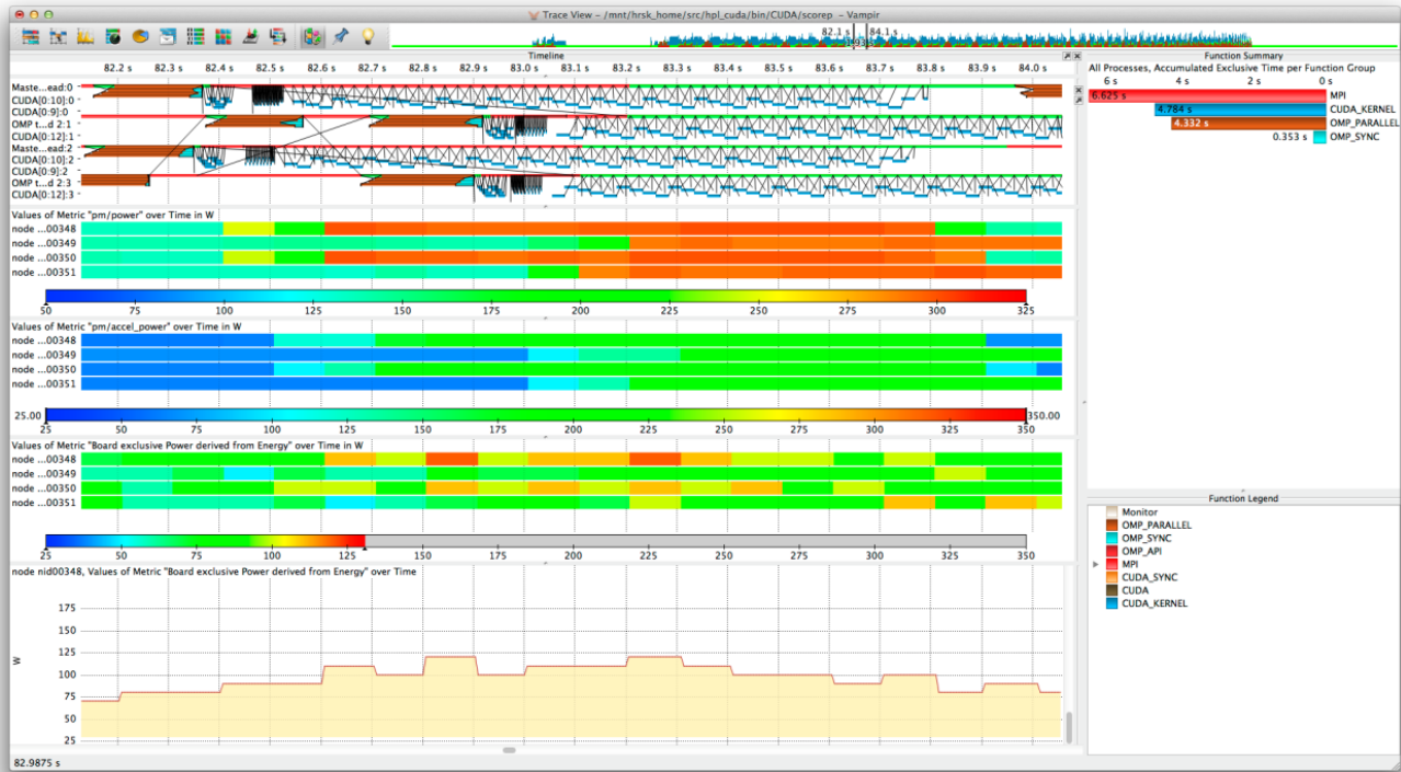
Figure 9. Colour-coded visualisation of HPL CUDA with Vampir. The topmost timeline shows the behaviour of the processes, threads, and CUDA streams over time for an interval of 2s. The second timeline displays the instantaneous node power over time. The third timeline displays the instantaneous graphic card power and the lowest timeline displays the board exclusive power without the graphic card derived from the energy for the first node nid00348 out of the four nodes.
