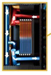
Liquid-to-liquid HEXs exchange heat between facilities liquid loop and server liquid loops. Facilities and server liquids are kept separate and never mix.
