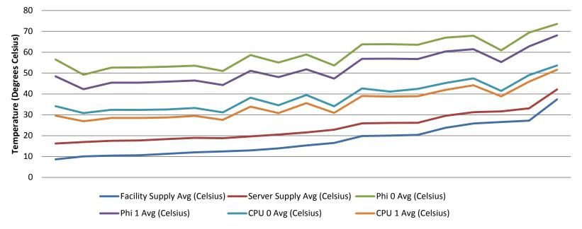
With average facility fluid temps of 37°C, internal (secondary) fluid loop temperatures were 42°C
