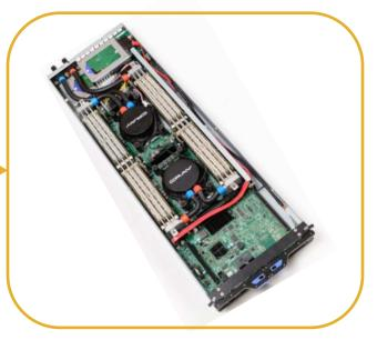
Pump/cold plate units atop CPUs (or GPUs) circulate liquid through blades and RackCDU, collecting heat and returning to RackCDU for exchange with facilities liquid.
