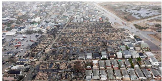
Figure 12. Over 80 homes were lost at Breezy Point in the Rockaways to fire alone caused by downed power lines and salt water.
