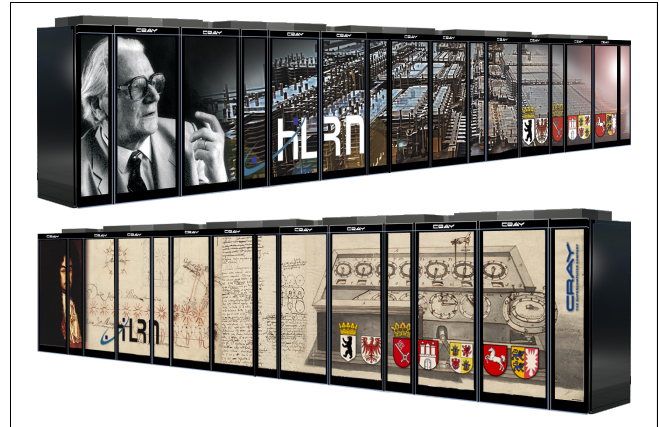
Figure 2. The Cray XC30 system “Konrad” in Berlin (top) in its final stage will comprise 10 cabinets whereas the XC30 system “Gottfried” in Hannover (bottom) will offer 9 cabinets and 64 additional external SMP nodes in total.
