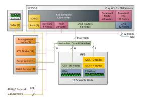
A combination of networking technologies will be used to bind these parts of the system together providing high performance integration and to make the system accessible. Data transfer between the storage subsystem and the compute and login nodes will be possible through FDR InfiniBand connections. A combination of 1 GigE and 40 GigE network connections will provide the integrated communications as well as performance connectivity for accessing the system.
