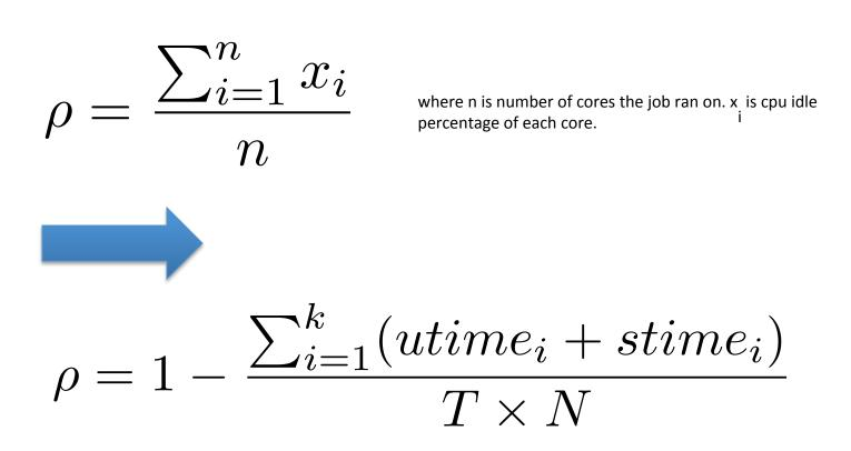
where k is the number of aprun, utime and stime are from the RUR taskstats plugin record with apid, T is the wall time elapsed for the whole job, N is the number of cores actually assigned to the job, sum up the values of ppn with the nid in array of allocated host names from job accounting information
