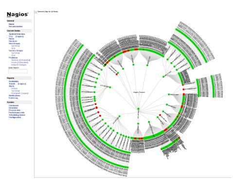
temperature gets out of range. The 500 power points are collected at 1 second interval. This power data includes data from the host all the way up to the building substation. Also being monitored is the UPS and all the power quality delivered at each stage. This Nagios map shows the PDU strips and their status.
