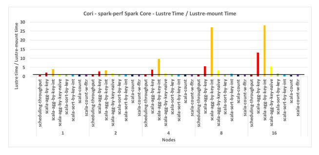
Figure 11. Slowdown of spark-perf Spark Core benchmarks on Cori with shuffle intermediate data stored on the Lustre filesystem instead of Lustre-backed loopback filesystems.
