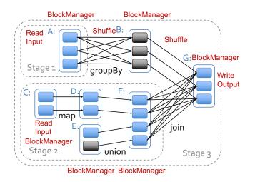
Figure 3. An example lineage showing the types of Disk I/O that can occur during each phase of the computation.
