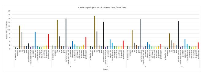
Figure 8. Slowdown of spark-perf MLLib benchmarks on Comet with shuffle intermediate data stored on the Lustre filesystem instead of local SSDs.
