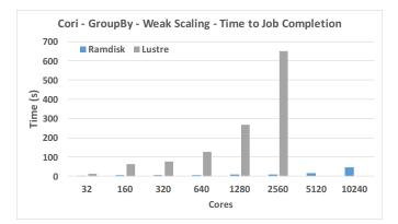
Figure 4. GroupBy benchmark performance (worst-case shuffle) on NERSC Cori, with shuffle intermediate files stored on Lustre or RAMdisk. Number of partitions in each case is  $4 \times cores$
