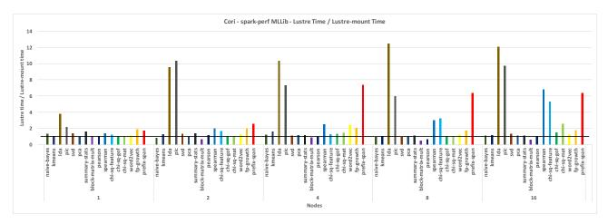
Figure 12. Slowdown of spark-perf MLLib benchmarks on Cori with shuffle intermediate data stored on the Lustre filesystem instead of Lustre-backed loopback filesystems.
