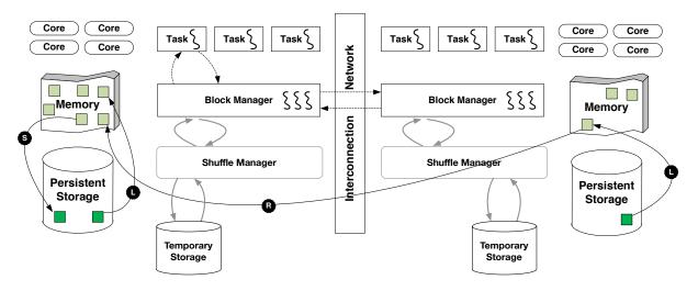
Figure 2. The storage infrastructure of Spark. Tasks request blocks from and store blocks to the BlockManager, which manages both memory and disk. The BlockManager communicates with the ShuffleManager to sort shuffle data and write shuffle data to temporary storage. Inter-node communication occurs through messages sent between BlockManagers.
