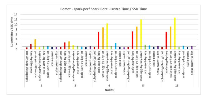
Figure 6. Slowdown of spark-perf Spark Core benchmarks on Comet with shuffle intermediate data stored on the Lustre filesystem instead of local SSDs.
