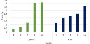
Figure 13. Weak scaling for the MLLib benchmarks most sensitive to shuffle performance on Cori with per-node loopback filesystems and on Comet with local SSDs.
