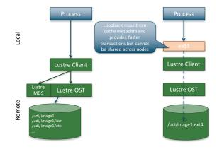
Figure 9. Shifter can mount node-local filesystems, keeping metadata operations local but preventing cross-node access.
