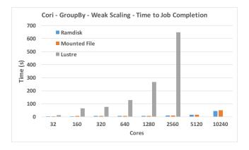
Figure 10. GroupBy benchmark performance (worst-case shuffle) on NERSC Cori, with shuffle intermediate files stored on Lustre, RAMdisk, or per-node loopback filesystems backed by Lustre files. Number of partitions in each case is  $4 \times cores$
