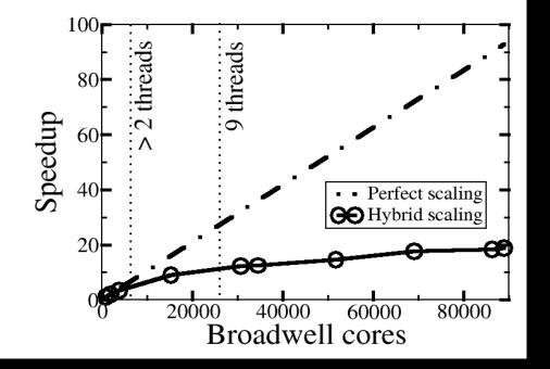
More than 2 threads required to avoid MPI-turnover at ~10k cores.
