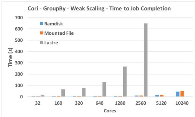
Figure 10. GroupBy benchmark performance (worst-case shuffle) on NERSC Cori, with shuffle intermediate files stored on Lustre, RAMdisk, or per-node loopback filesystems backed by Lustre files. Number of partitions in each case is  $4 \times \text{cores}$
