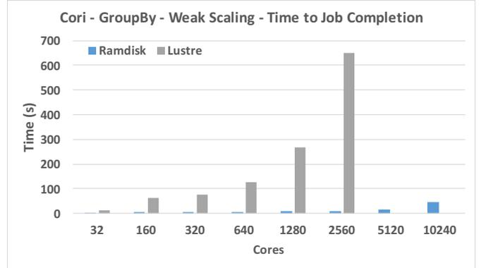
Figure 4. GroupBy benchmark performance (worst-case shuffle) on NERSC Cori, with shuffle intermediate files stored on Lustre or RAMdisk. Number of partitions in each case is  $4 \times cores$
