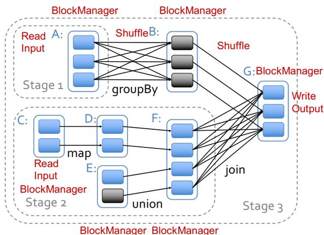
Figure 3. An example lineage showing the types of Disk I/O that can occur during each phase of the computation.
