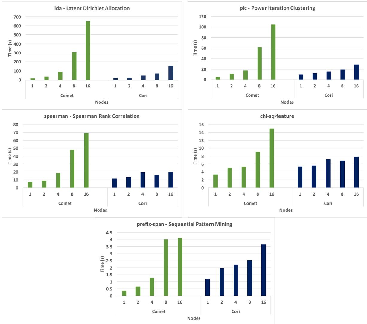
Figure 13. Weak scaling for the MLLib benchmarks most sensitive to shuffle performance on Cori with per-node loopback filesystems and on Comet with local SSDs.
