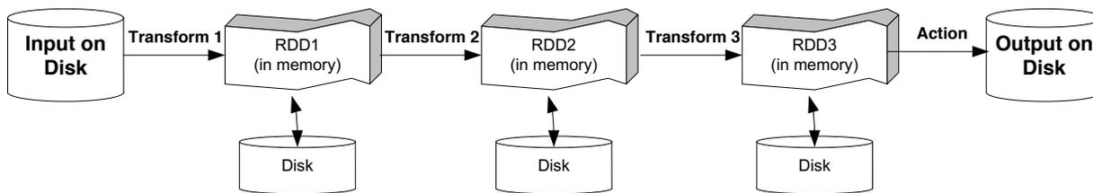
Figure 1. A chain of RDDs produced by applying transformations to an input dataset or predecessor RDDs. An action at the end of the chain triggers deferred computation.
