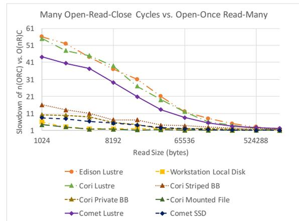
Figure 7. Slowdown from performing open-per-read rather than single-open many-reads for reads of different sizes on various filesystems on Edison, Cori, Comet, and a workstation with local disk. The penalty is highest for the Lustre filesystems.
