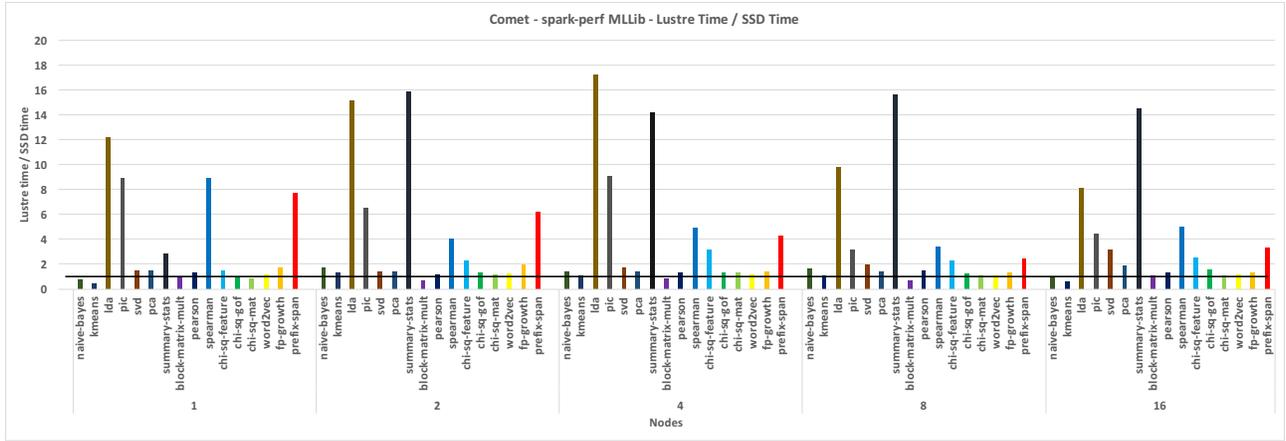
Figure 8. Slowdown of spark-perf MLLib benchmarks on Comet with shuffle intermediate data stored on the Lustre filesystem instead of local SSDs.
