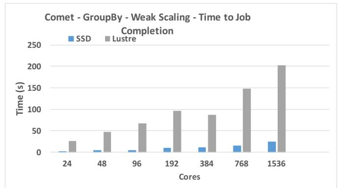
Figure 5. GroupBy benchmark performance (worst-case shuffle) on SDSC Comet, with shuffle intermediate files stored on Lustre or local SSD. Number of partitions in each case is  $4 \times cores$
