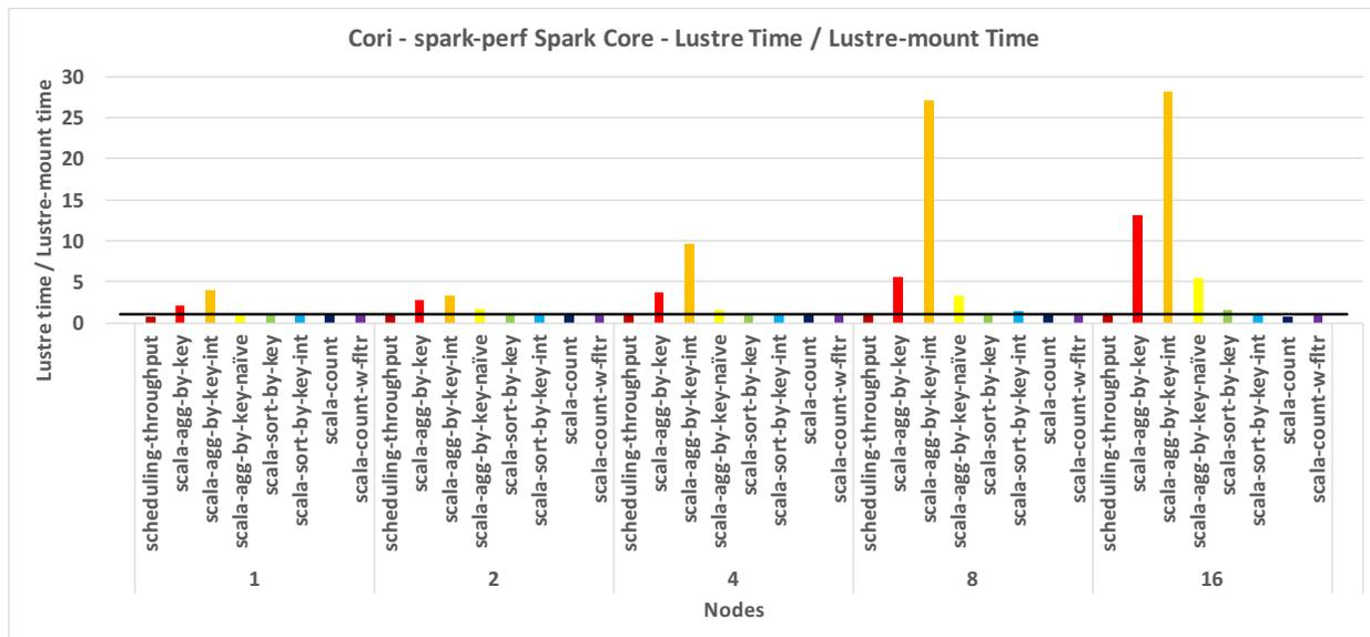
Figure 11. Slowdown of spark-perf Spark Core benchmarks on Cori with shuffle intermediate data stored on the Lustre filesystem instead of Lustre-backed loopback filesystems.
