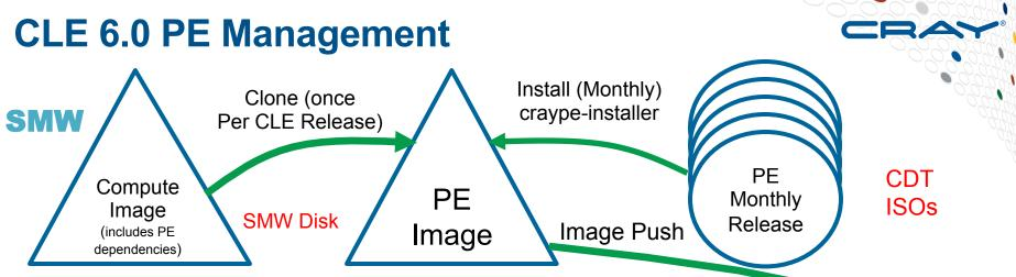
Once installation has completed (including PE third party software), PE image root pushed to the boot node:
