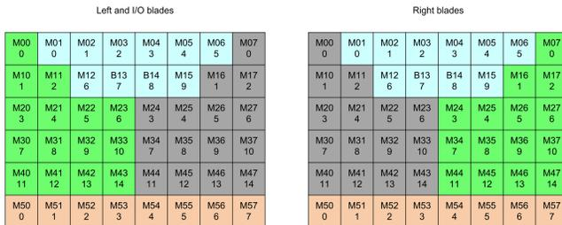
Figure 2: Aries tiles with color denoting one of Orange (NIC electrical), Green (intra-chassis electrical), Black (intra-group electrical), and Blue (inter-group optical) (From [8]).
