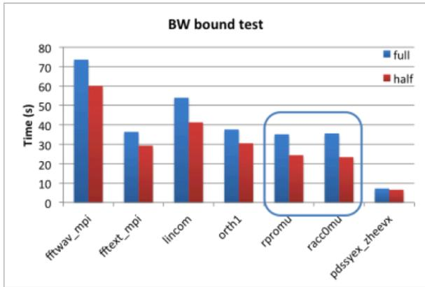
Figure 10. The VASP run time breakdown over the top subroutines when running on the fully packed (blue) and half-packed (red) nodes. The tests were done on an Intel Xeon E5-2697 v3 node and used the test case PdO@Pd-slab. When running on half packed nodes, the memory bandwidth available for each task is twice as much as it is when running on fully packed nodes. This experiment was designed to test if an application code is bandwidth bound.
