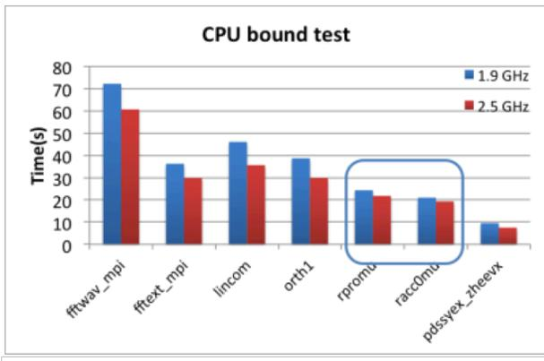
Figure 11. The VASP run time breakdown over the top subroutines when running at the clock speeds of 2.5 GHz, and 1.9 GHz on an Intel Xeon E5-2697 v3 node. The test case used was PdO@Pd-slab, and this experiment was designed to test if the code is CPU bound.
