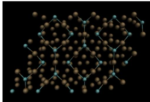
Figure 7. The benchmark test case used in profiling the MPI/OpenMP hybrid VASP code (the development version up-to 9/29/2015). The test system contains 150 Palladium (Pd) atoms and 24 Oxygen atoms (O) (denoted as PdO@Pd-slab hereafter), 1644 electrons in 1024 bands, and 33967 planewaves per band. The RMM-DIIS iteration scheme was tested, and it was executed over multiple bands simultaneously.
