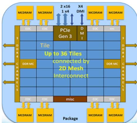
Figure 1. Intel KNL overview (source: Intel). Each KNL processor will have 72 cores (288 threads) at <1.4 GHz, 96GB DDR4 memory utilizing six 16GB DIMMs at 2400GHz, and a 16 GB MCDRAM with about 5x memory bandwidth of the DDR4 memory. Processor cores will be interconnected in a 2D mesh network with two cores per tile (36 tiles in total), with a 1-MB L2 cache shared between two cores in a tile, with two 512 bit vector processing units per core, and with multiple NUMA domain support per socket.
