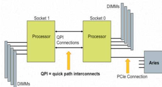
Figure 2. Edison compute node diagram (source: Cray). Each Edison compute node has two 12 cores Ivy Bridge processors (24cores/48 threads per node) at 2.4 GHz. Each node has 64GB DDR3 1866 MHz memory utilizing eight 8 GB DIMMs. Each core has its own L1 and L2 caches, with 64 KB (32 KB instruction cache, 32 KB data) and 256 KB, respectively; a 30-MB L3 cache shared between 12 cores on the processor (socket). Stream TRIAD bandwidth per node is 103 GB/s.
