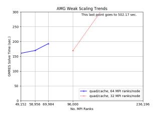
Figure 5. AMG weak scaling for *quad/cache* sized from SSP problem; this is a semilog plot where the x axis is logarithmic with a base of 2.
