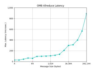
Figure 9. MPI Allreduce latency on 1,024 nodes.
