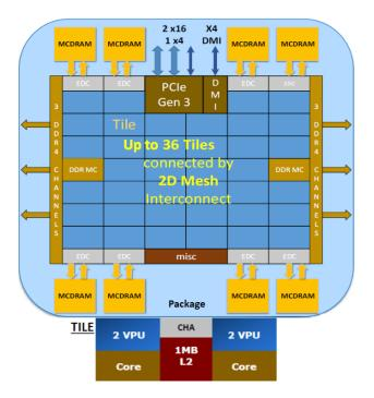
Figure 2. Diagram of Trinity's KNL node architecture.
