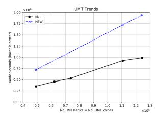
Figure 6. UMT scaling comparison between HSW and KNL for "large" MPI rank counts.
