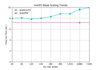
Figure 4. MiniFE weak scaling for quad/cache sized from SSP problem; this is a semilog plot where the x axis is logarithmic with a base of 2.
