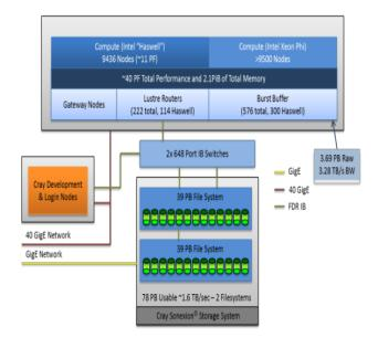
Figure 1. High-level diagram of Trinity's architecture.
