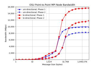
Figure 8. OMB node-to-node MPI bandwidth.
