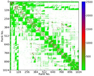
Figure 3. Heat map of total number of point-to-point (p2p) calls for "R3" Nalu simulation initialization and a single time step on 1,024 MPI ranks (16 nodes with 64 ranks per node).
