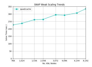
Figure 7. SNAP weak scaling for *quad/cache* sized from SSP problem; this is a semilog plot where the x axis is logarithmic with a base of 2.
