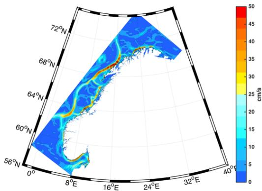
*Figure 2: Map showing the extension of the NorKyst800 model. The colors denote the long-term average of surface current speed. The mean current patterns are mainly directed northwards, and the color scale denotes speed in cm/s.*
