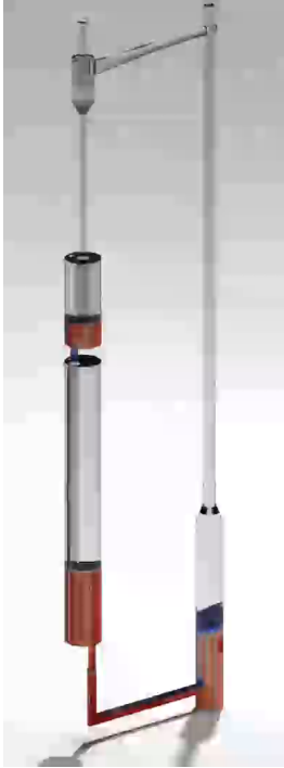
2016 Two-Fluid-Model of Pilot-scale Reactor Particles treated as a granular fluid
