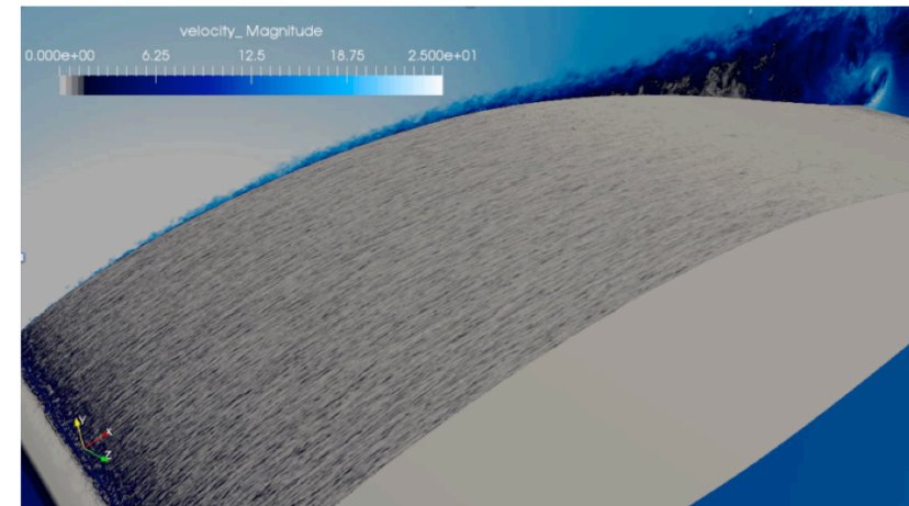
Wall-resolved LES study of a turbine-blade section; 1.6 billion cells
