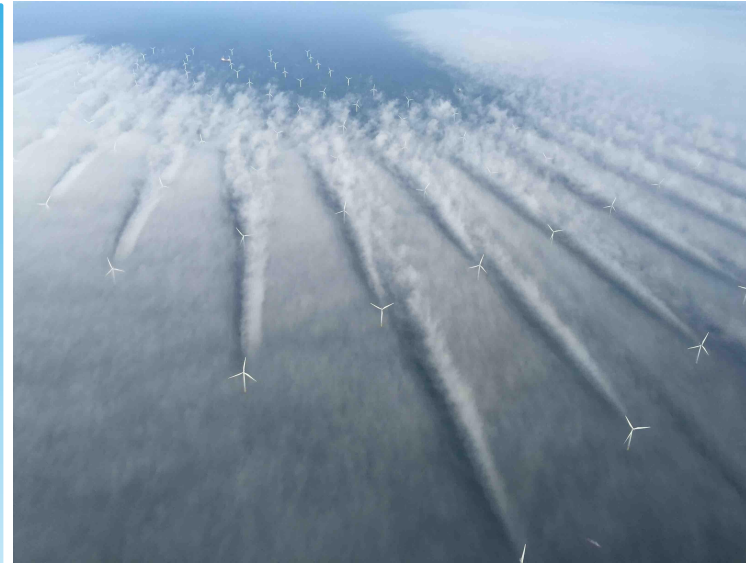
Horns Rev wind farm in the eastern North Sea off of Denmark; wake dynamics highlighted by sea smoke
