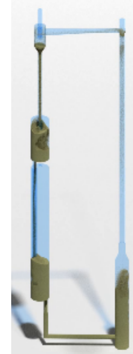
2026 CFD-DEM of Pilot- scale reactors Particles are individually tracked
