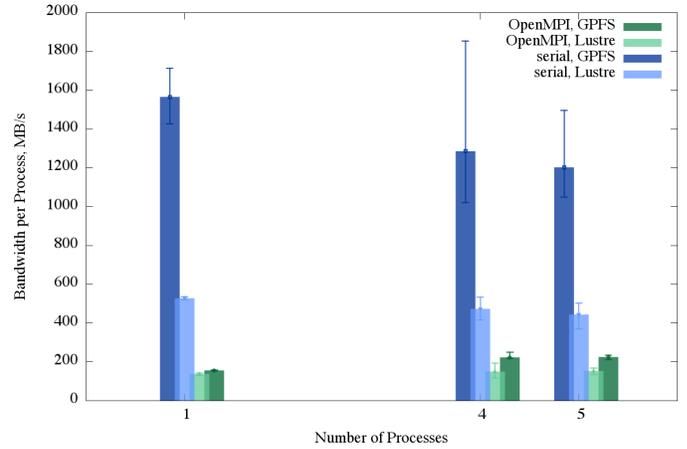
Fig. 1. Parallel write performance on a cluster at Diamond Light Source (DLS) facility for appending 2D image frames to a 3D dataset. The performance of executing serial writes per process ranges from five to ten times faster than writing to a single file [12].
